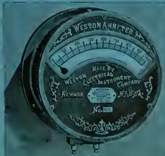
Weston "Round Pattern" Ammeter, Type F.
