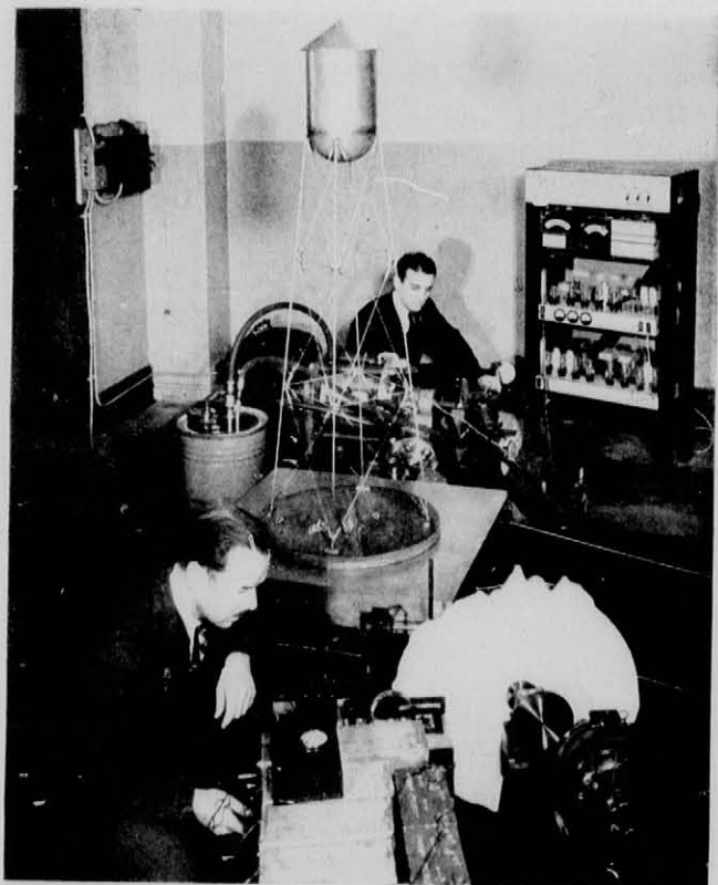
Testing water tanks with synthetic earthquakes. The white shadograph in the right foreground represents an actual quake, and through an electrical system causes the table upon which the tank stands to move as the ground did in the actual quake
