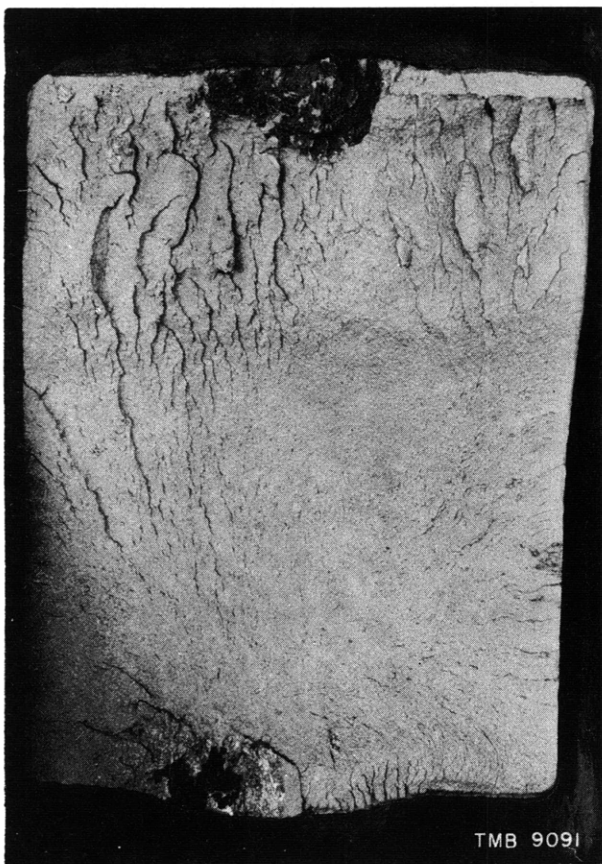
Figure 5 - View of Anchor after Tensile Loading Test
