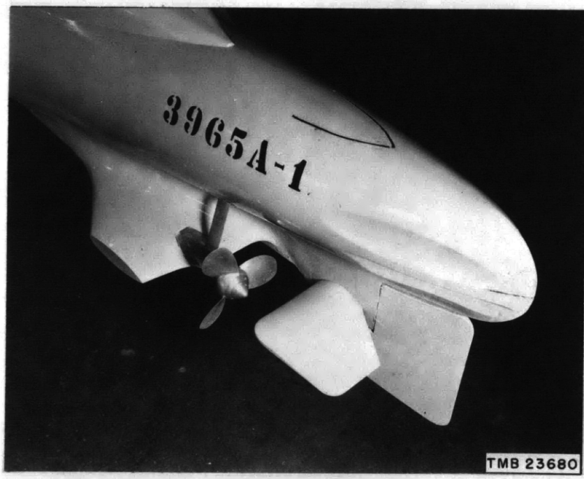
Figure 2 - Stern of a Model of a Submarine of the SS487 Class with Stabilizing Planes
