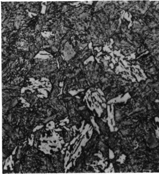
Figure C2a – 14 Percent Bainite – 86 Percent Martensite 875 F – 152 Sec
