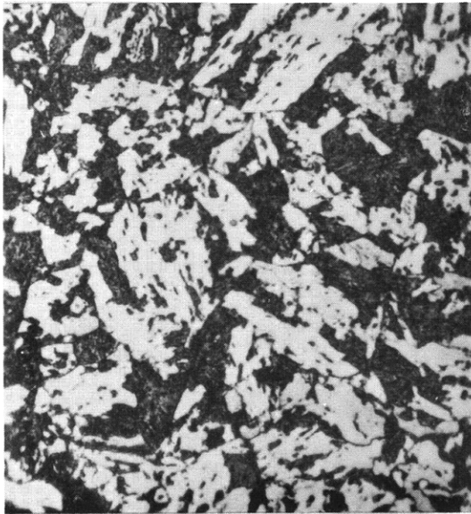
Figure C1c – 54 Percent Bainite – 46 Percent Martensite 875 F – 1600 Sec
