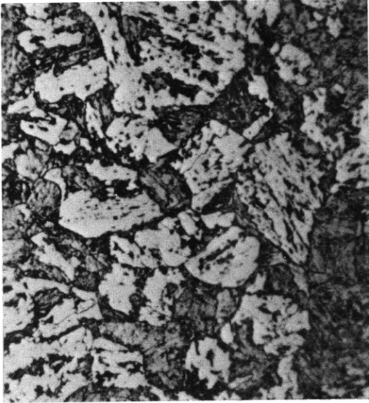
Figure C4a – 50 Percent Bainite – 50 Percent Martensite 875 F – 1600 Sec
