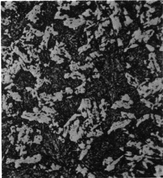
Figure C3c – 41 Percent Bainite – 59 Percent Martensite 875 F – 1600 Sec
