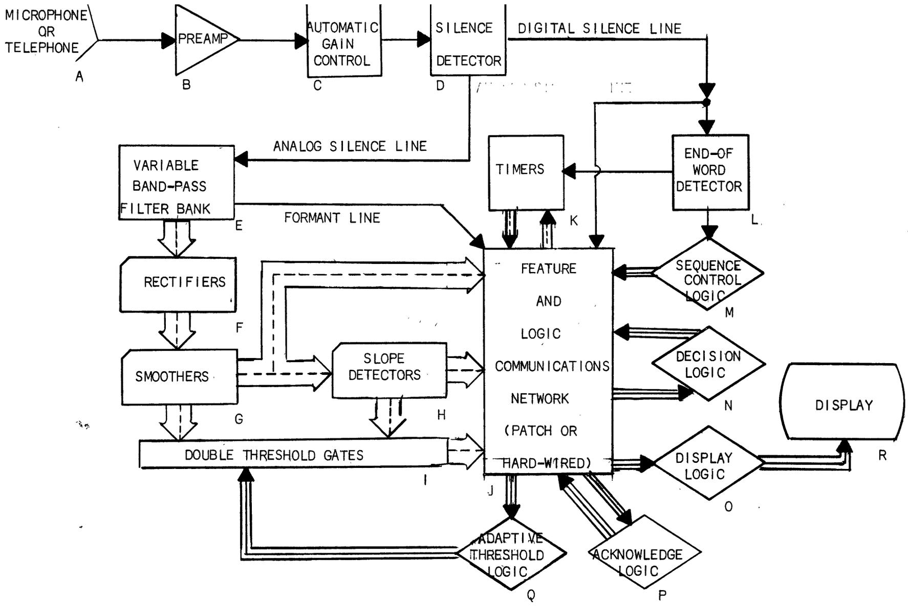
Figure 1 - Slope/Intensity Detection System for Speech Recognition
