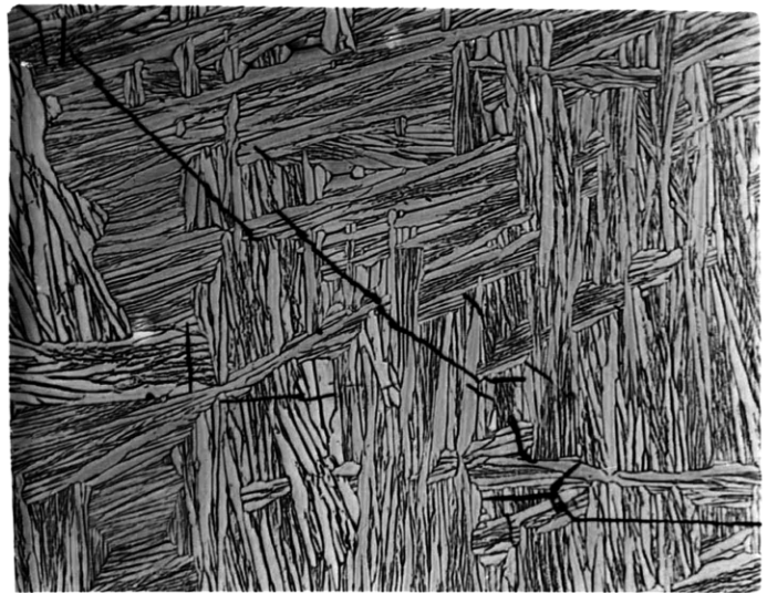
Figure 18 - Crack Network in a Partially Failed Ti-7Al-2Cb-1Ta Specimen in the Beta-Rolled and Beta-Annealed Condition
