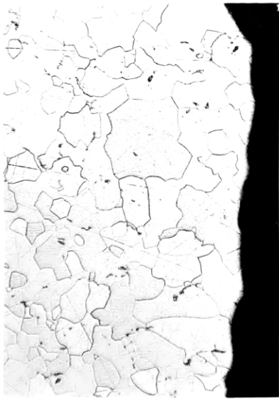
Item (a) Fatigue Cracked Zone
