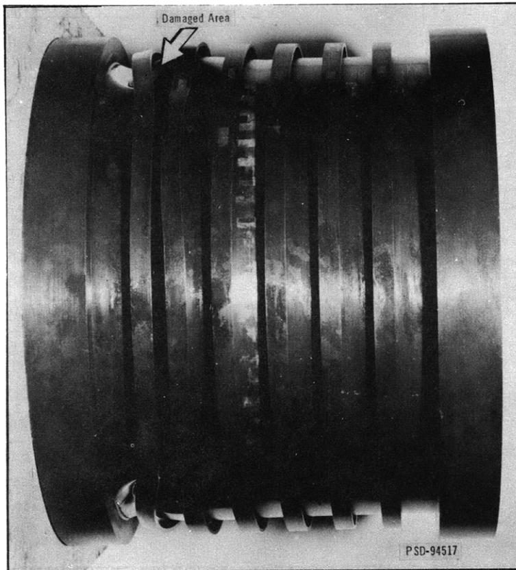
Figure 5 – Collapse of Model 1
