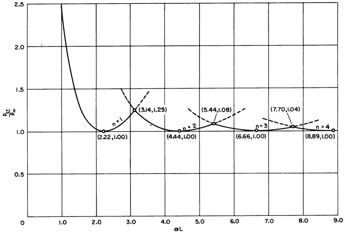
Figure 2 – Curves for Axisymmetric Buckling of Cylinders under External Hydrostatic Pressure
