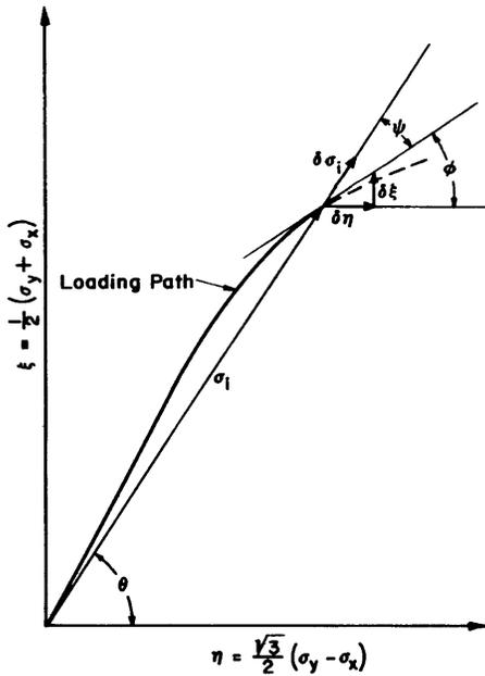
Figure 7 – Loading Path Diagram for Determination of Angle  $\psi$
