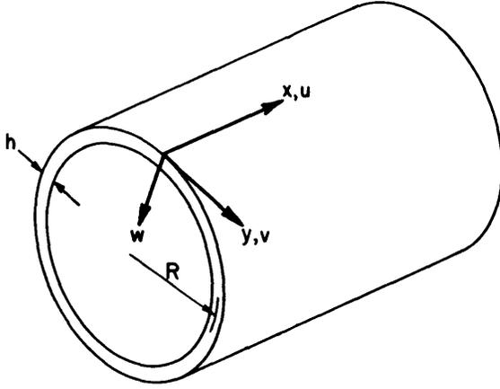
Figure 1 – Coordinates and Components of Displacement
