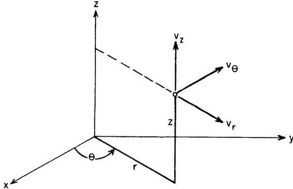
Figure 9 - Coordinate System for Rotational Symmetric Flows
