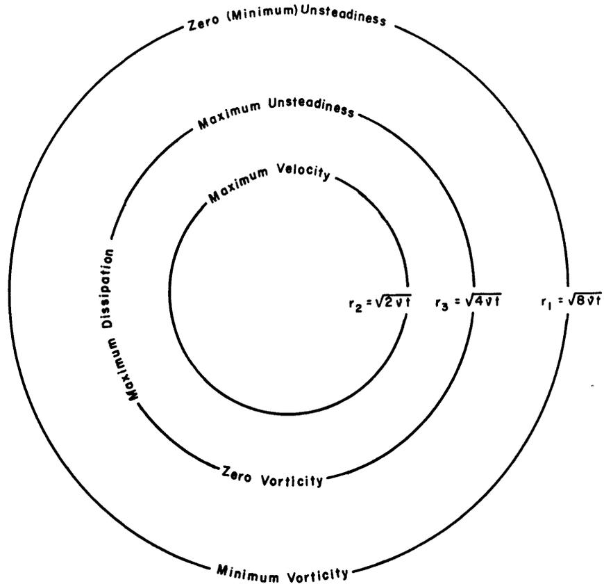
Figure 7 - Characteristics of a Circular Eddy
