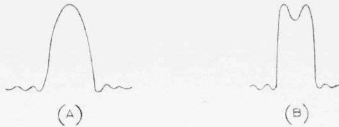
FIGURE 18. EFFECT OF BANDWIDTH ON PULSE SHAPE (A) BANDWIDTH TO \frac{1}{8} (B) BANDWIDTH TO \frac{2}{8}
