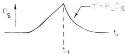
FIGURE 46. WAVEFORM OF e_s PRODUCED BY CIRCUIT OF FIGURE 45.
