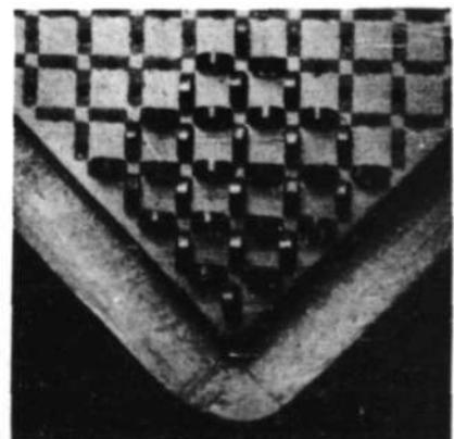
Corner of plastic form, showing 36 cores in correct orientation in the pockets. Air is sucked through hole in bottom of each core pocket at a high rate during core positioning and at a lower rate during wiring of a 4,096-core plane
