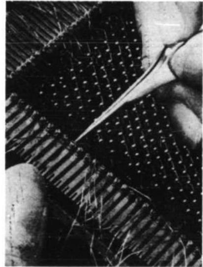
Method of using tweezers to aid in placing second loop of a Y wire in slot of sub-miniature lug on etched-wiring frame of memory plane. Between 2 and 3 hours are required to make these connections, straighten out lines of mat and clip off surplus wire
