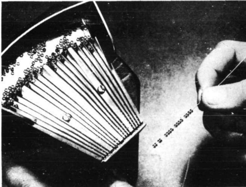
Older technique required that cores be threaded on a long needle and wired into large frame manually. The only significant mechanized aid was the counter-threader shown here, which presented 16 cores at a time to operator. Cores gradually turn to vertical position as they slide down contoured chutes to threading position at bottom
