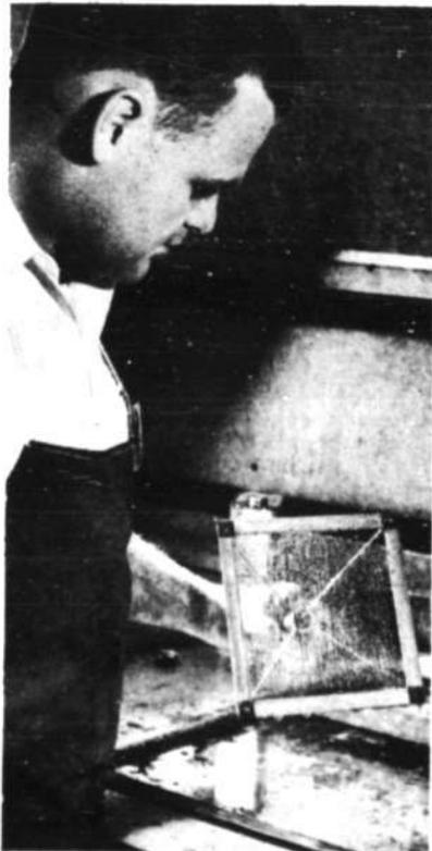
After dip soldering each of the four edges of the plane in turn, unit is ready for inspection and test
