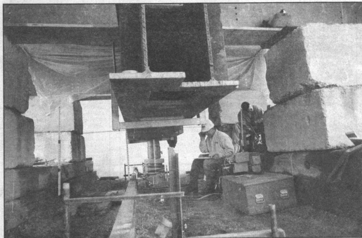
Inside the 200-ton test block, Rusty Brown (center) and Lance Mugford (far right) monitor test equipment calculating the load on the column and footing. Photo by Donna Coveney
