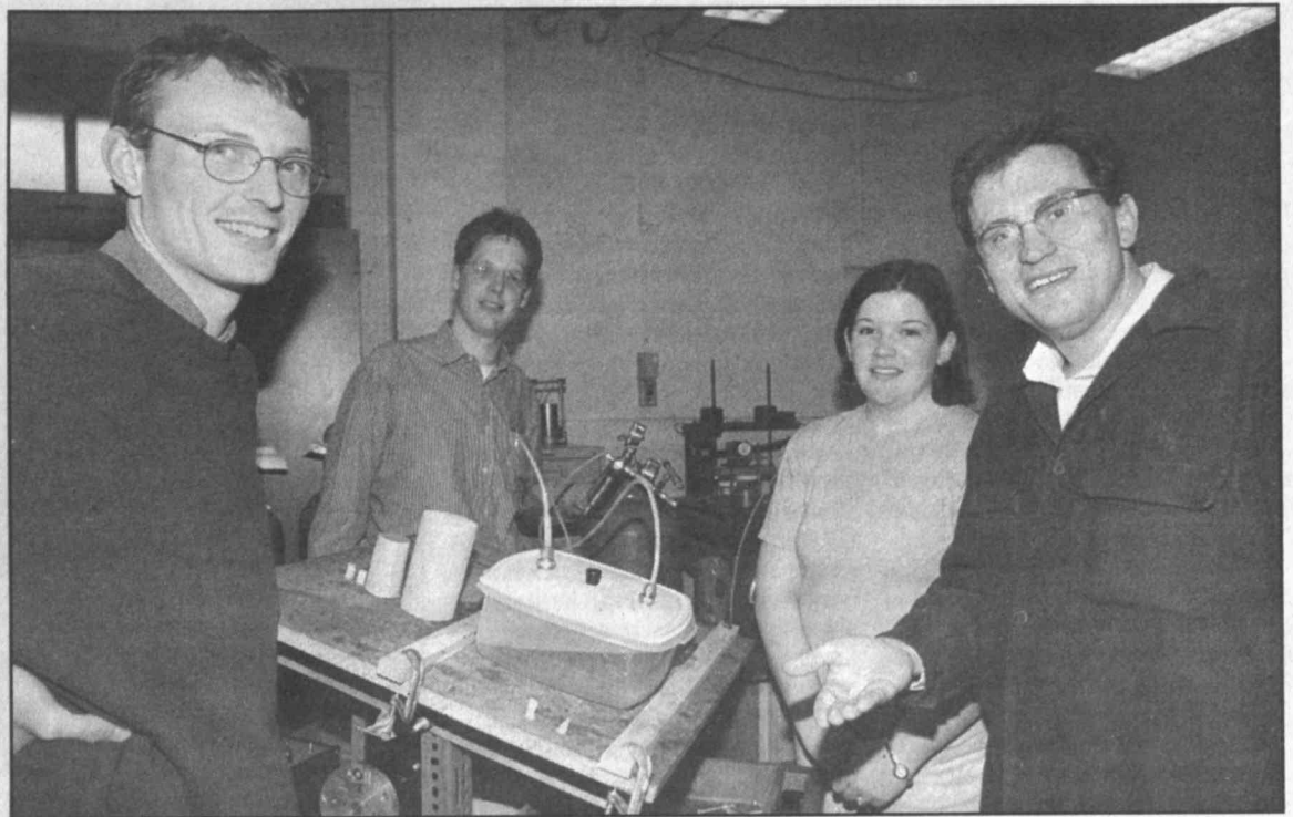
Gathered around the table they developed to test and predict the stability of concrete over long periods of time are (left to right) postdoc Marc Mainguy; graduate student Franz Heukamp; Jennifer Butz, a junior in civil engineering; and Professor Franz Ulm. Concrete samples are treated on this seesawing table, immersed in the container at right. To the left are examples of concrete before immersion. Photo by Donna Coveney
