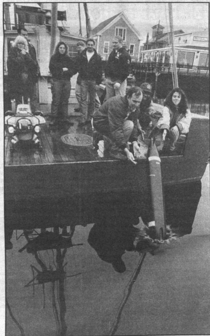
Christopher von Alt of WHOI, Khary Bridgewater, '95, and Claudia Rodriguez pitch Remus, a lightweight AUV (automated underwater vehicle), off the WHOI research vessel Asterias into Eel Pond in Woods Hole as part of a two-week field engineering lab required for their master's degree in the Ocean Engineering department. Among those looking on are Ocean Engineering Professor Judith Kildow and graduate students Jon Grant, Nicole Suoja, Erik Burian and Joseph Curcio.
