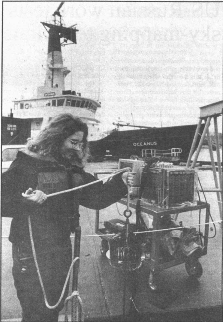
Nicole Suoja, a graduate student in Ocean Engineering, lowers an instrument to measure waves (wave gauge) into the water off a dock at Woods Hole. The instrumentation measures directional distribution and size of short sea waves.
