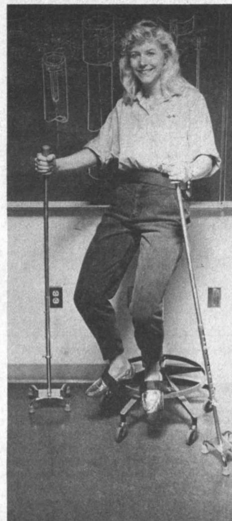
MIT senior Penny Plummer demonstrates her "standup mobility device," intended to enable wheelchair-bound persons to move about in a near-standing position in classrooms, offices and homes.
