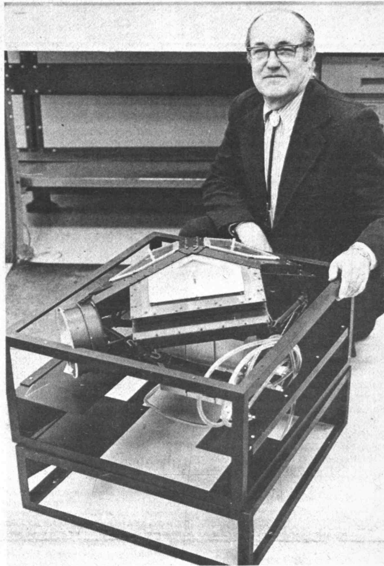
Professor Herbert S. Bridge is shown here with a prototype of the instrument aboard Voyager 1 which is measuring the solar wind near Jupiter. —Photo by Calvin Campbell
