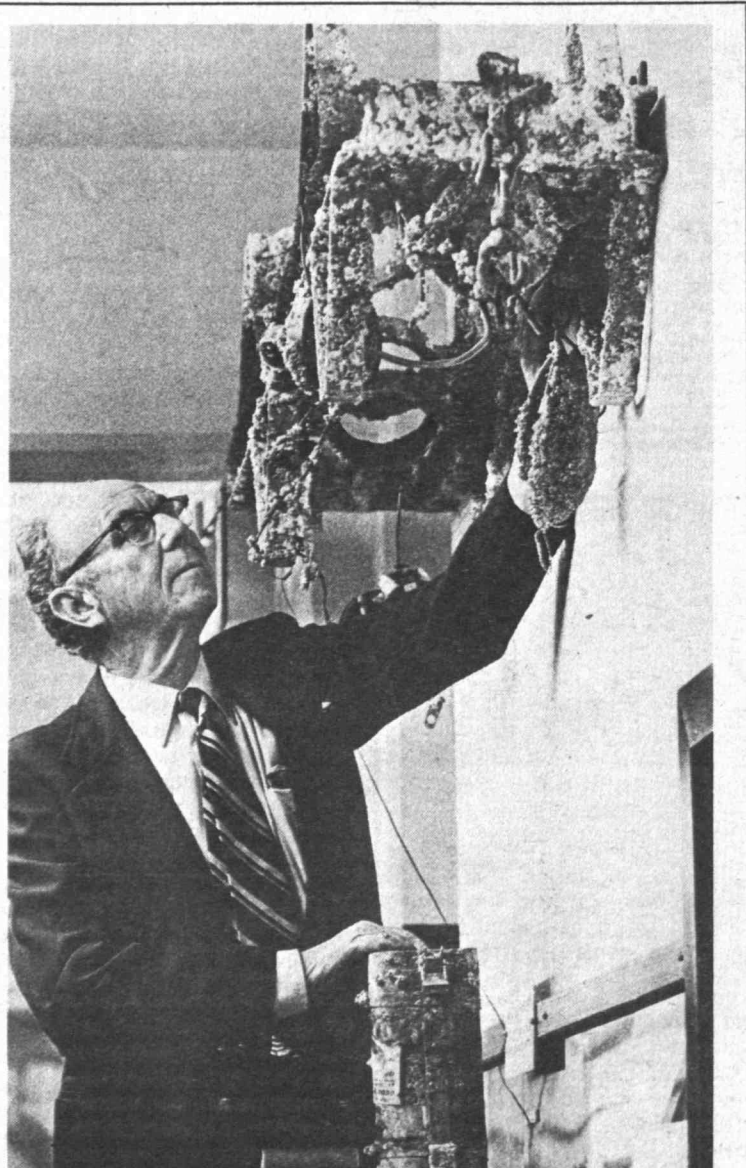
FROM OCEAN BOTTOM TO DOC'S WALL—An undersea camera and strobe, raised from the wreck of the Civil War ironclad Monitor , has been mounted on the wall of Strobe Alley whose leading citizen is Professor Harold E. (Doc) Edgerton. The camera/strobe unit was lowered in 1973 to take pictures of the Monitor , which sank in a gale off Cape Hatteras. It lodged in the central portion of the ship, but was recovered last summer during another expedition to the famed warship.
