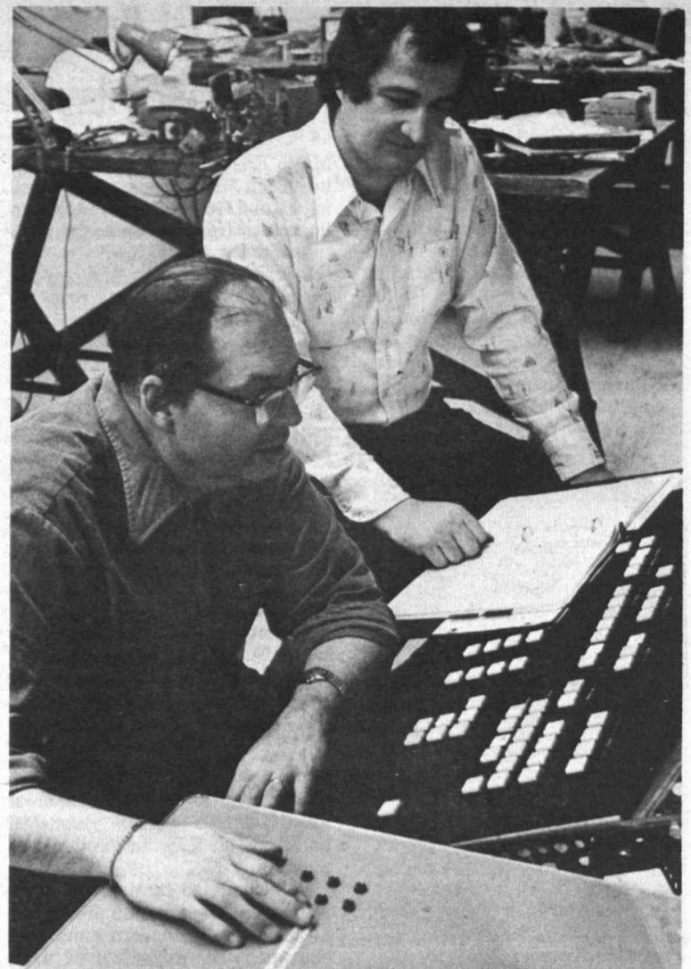
A BLIND PERSON'S alternative to a computer terminal's video display has been developed at the MIT Sensory Aids Evaluation and Development Center. Dr. Derek Rowell, rear, director of the center, said the device is expected to expand job opportunities for the blind. George Dalrymple, engineer at the center, tests with his fingers the pins that provide the Braille display. The computer terminal is a mock-up of the Bell System's Traffic Service Position System. A blind telephone operator will be trained to use the MIT device with the TSPS at Southwestern Bell Telephone Co. in Little Rock, Ark., where Dalrymple is installing the Braille-pin equipment.
