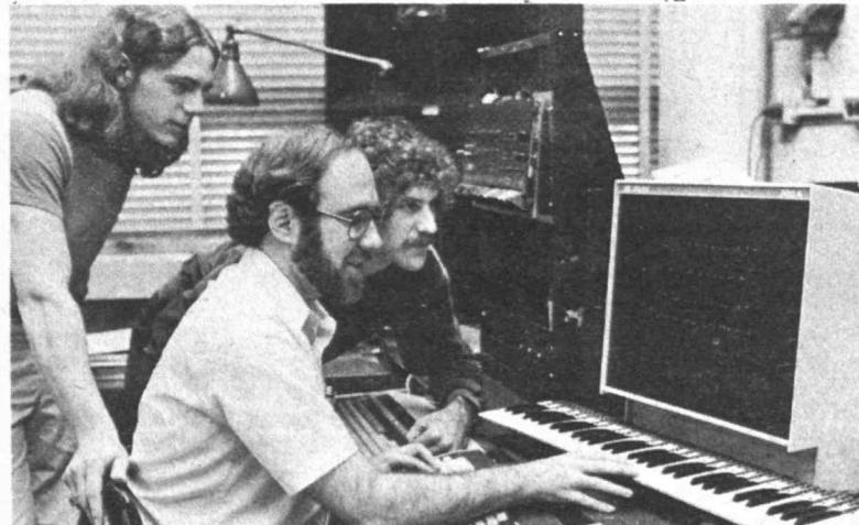
MUSICAL COMPUTER—Anthony Lake, Richard Steiger and Carl Howe "talk music" with a computer-based system that includes an organ keyboard input, display of standard music notation on the scope, hard copy music print-out, and digital synthesis of the sound.
