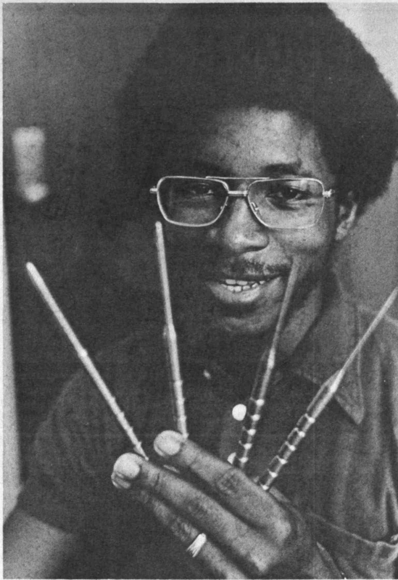
Woodrow Whitlow holds a series of aerodynamic models, representing different shapes of the forebodies of supersonic airplanes, which he used in his prizewinning research. Mr. Whitlow studies how shock waves from the shapes were affected by changes in air pressure.
