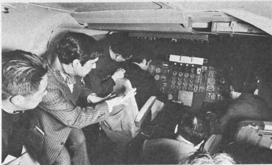
SKY DISPLAY —Interpreter (second from left) helps explain an experimental aircraft cockpit display system to editors from the People's Republic of China who toured the MIT Electronic Systems Laboratory last week. The cockpit display, part of a research program on air safety, is designed to show airliner pilots where other planes are with respect to his position in the vicinity of an air terminal.
