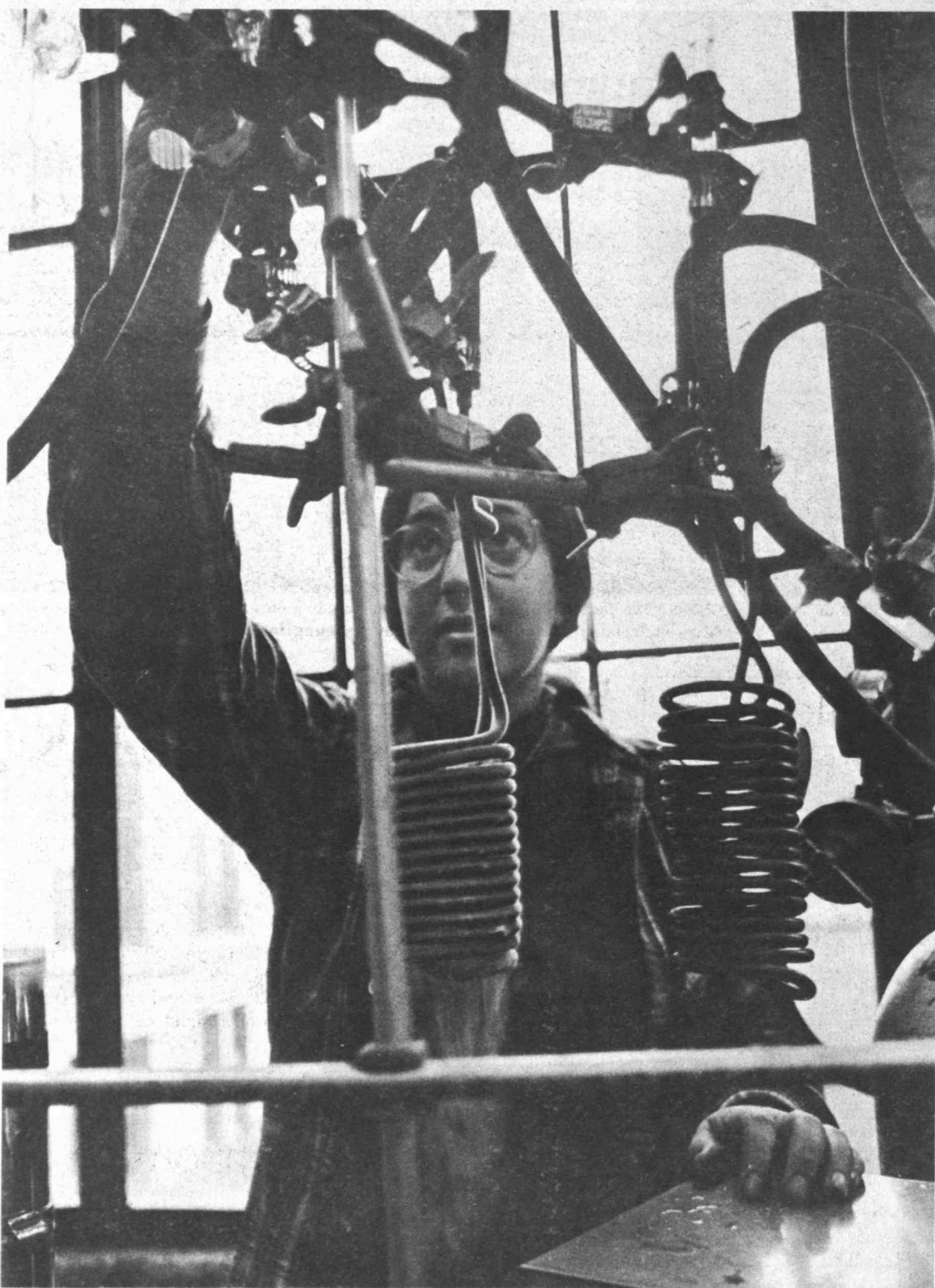
Shown above is Paula Elster, a junior in chemistry from Palo Alto, California, measuring mutual diffusion coefficients of helium and oxygen in a chemistry laboratory in Building 4.
