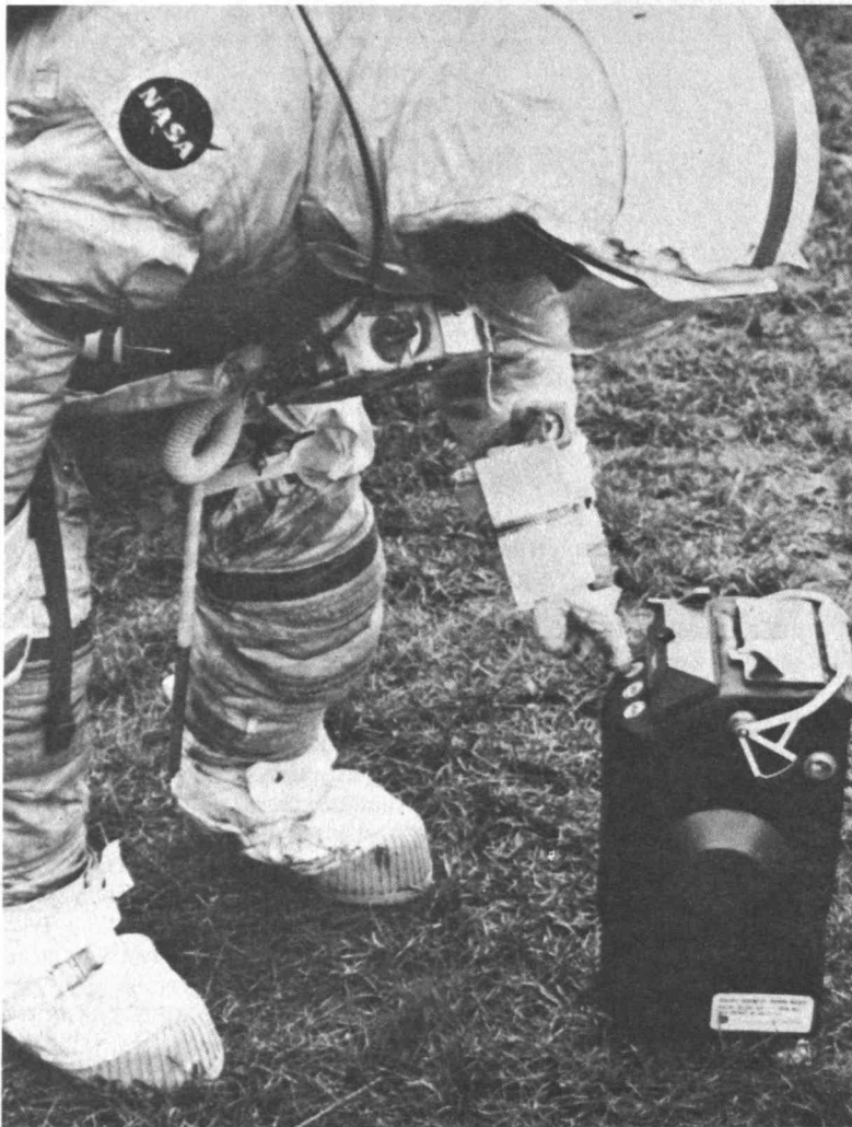
Astronaut Eugene Cernan checks out the traverse gravimeter, a new instrument designed and developed by the Draper Laboratory. The gravimeter will be used on the Apollo 17 Mission to obtain information for a lunar gravity profile.
