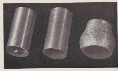
Test specimens of Cerrobend. Left, before load test; center, after 5650-lb. load at -320 F.; right, after 5650-lb. load without cooling
