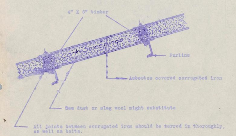
GROSS-SECTION OF BAGHOUSE ROOF SHOWING SUGGESTED METHOD OF HEAT INSULATION
