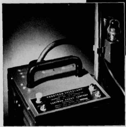
The Photoelectric Trip Unit clamps to the stand above the power unit. The photocell discharges a second lamp from the flash of the first. Any number of lamps, so equipped, can be flashed simultaneously. Note the few controls grouped on the name plate of the Kodatron Speedlamp.
