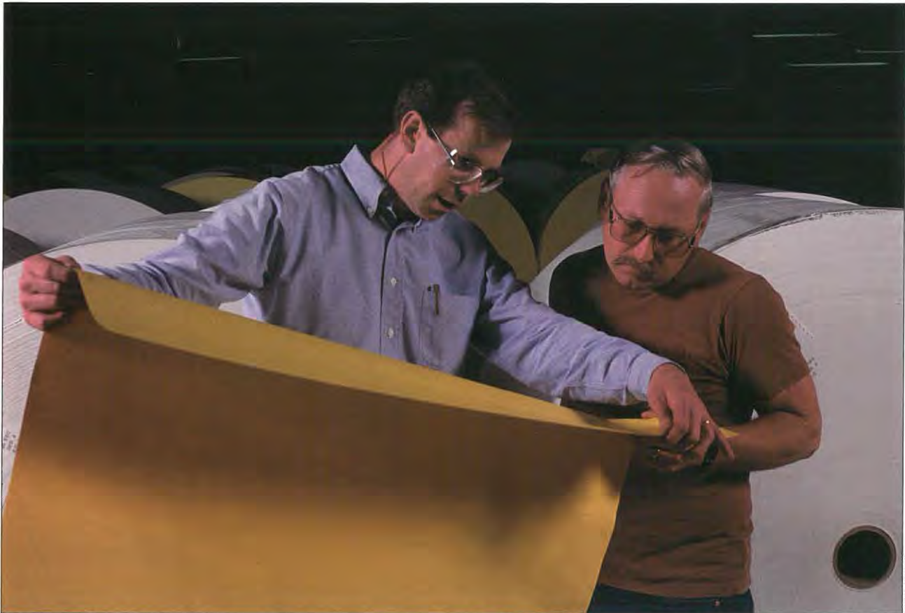
Tim Loucks '90 (l) confers with Tom Tubbs, sheeter operator (r), about the quality of a finished sheet of 50-lb offset printing paper at International Paper's Ticonderoga Mill.
