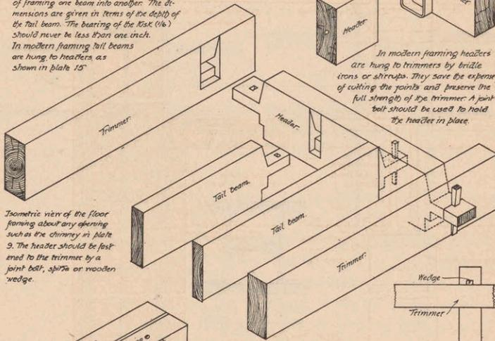
Isometric view of the floor framing about any opening such as the chimney in plate 9. The header should be fastened to the trimmer by a joint bolt, shroups or wooden wedge.
