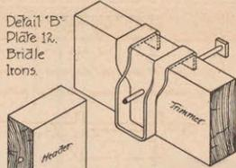
In modern framing headers are hung to trimmers by bridle irons or shroups. They save the expense of cutting the joints and preserve the full strength of the trimmer. A joint bolt should be used to hold the header in place.
