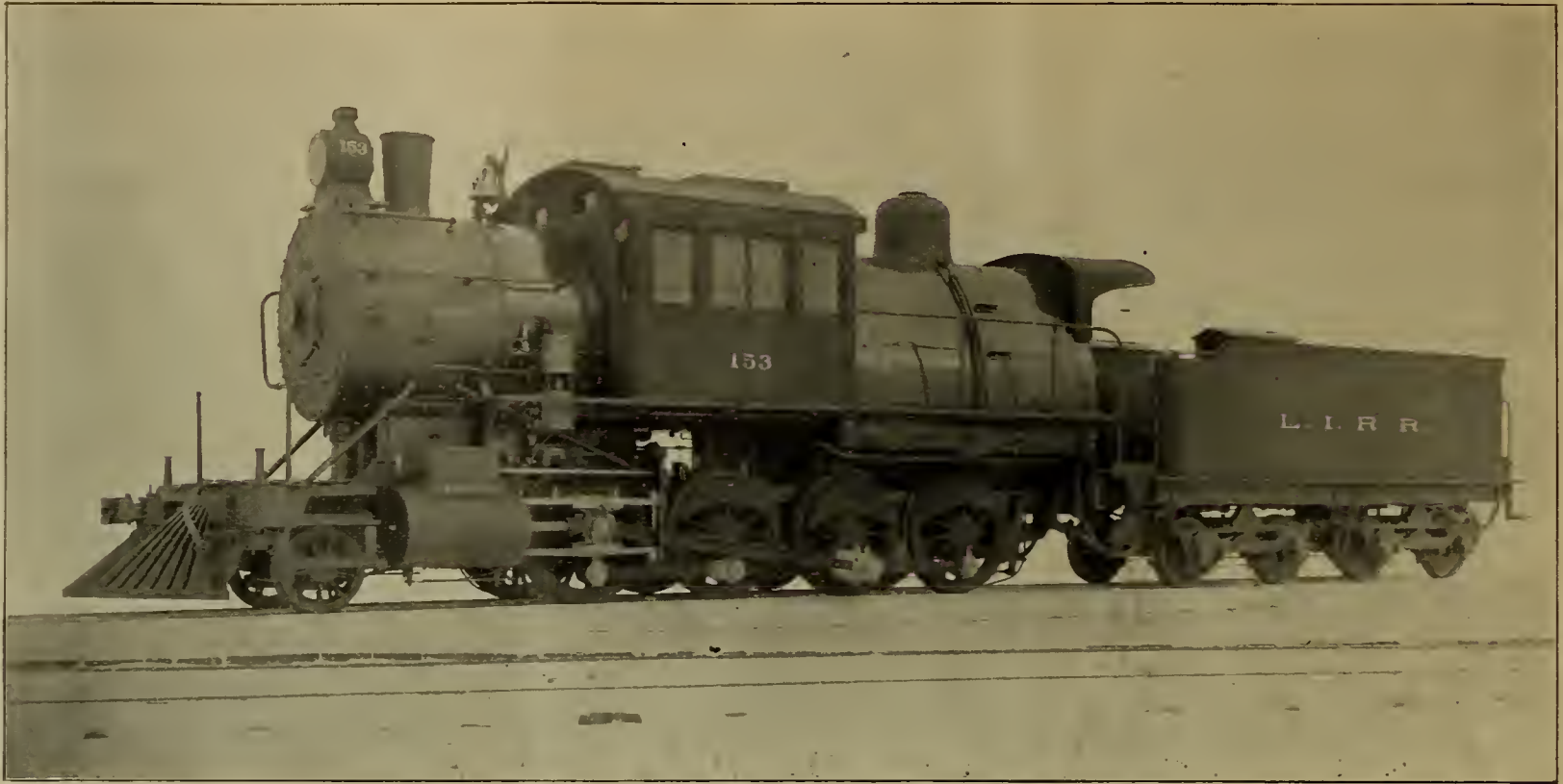
CONSOLIDATION LOCOMOTIVE—LONG ISLAND RAILROAD. Built by Brooks Locomotive Works.
