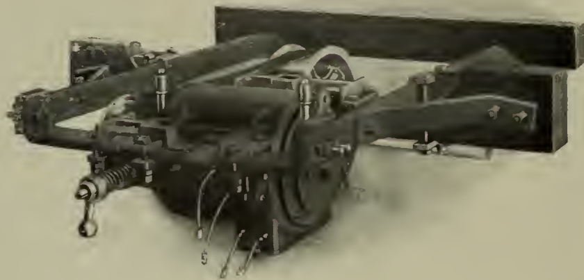
FIG. 8.—VIEW OF GENERATOR AND METHOD OF SUSPENSION IN THE SYSTEM OF THE BLISS ELECTRIC CAR LIGHTING COMPANY, OF MILWAUKEE, WIS.
