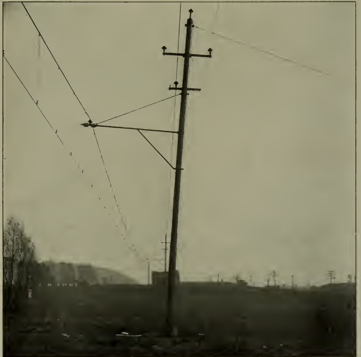
FIG. 3.—THE POLE WAS DEFLECTED AS HERE SHOWN UNDER A STRAIN OF 2050 POUNDS AT THE TOP, EXERTED AT A DISTANCE OF 125 FEET
