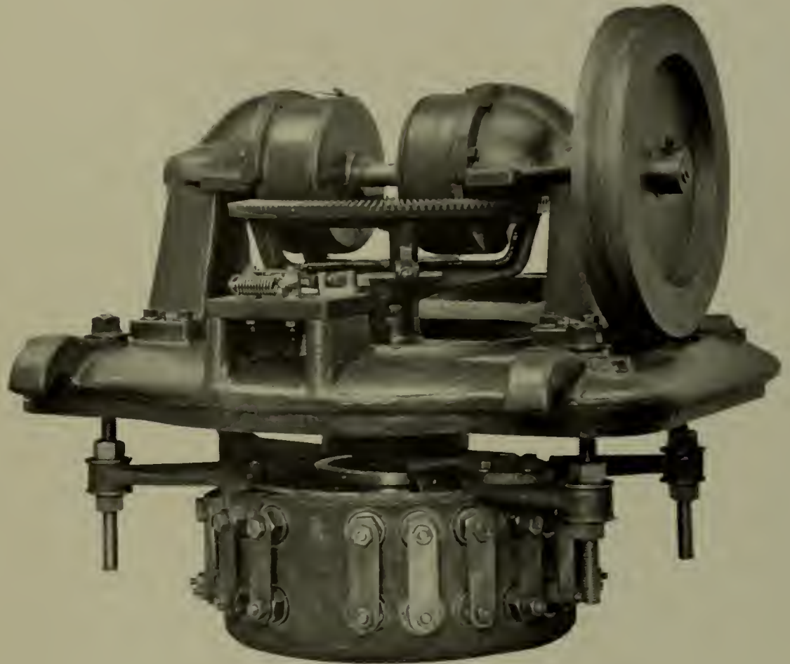
FIG. 7.—COVER OF THE SWITCH-TYPE REGULATOR WITH CONTROLLING MECHANISM
