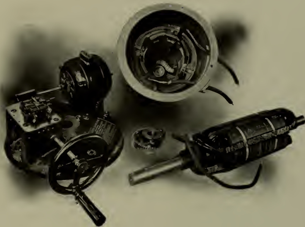
FIG. 15.—PARTS OF AN INDUCTION REGULATOR
