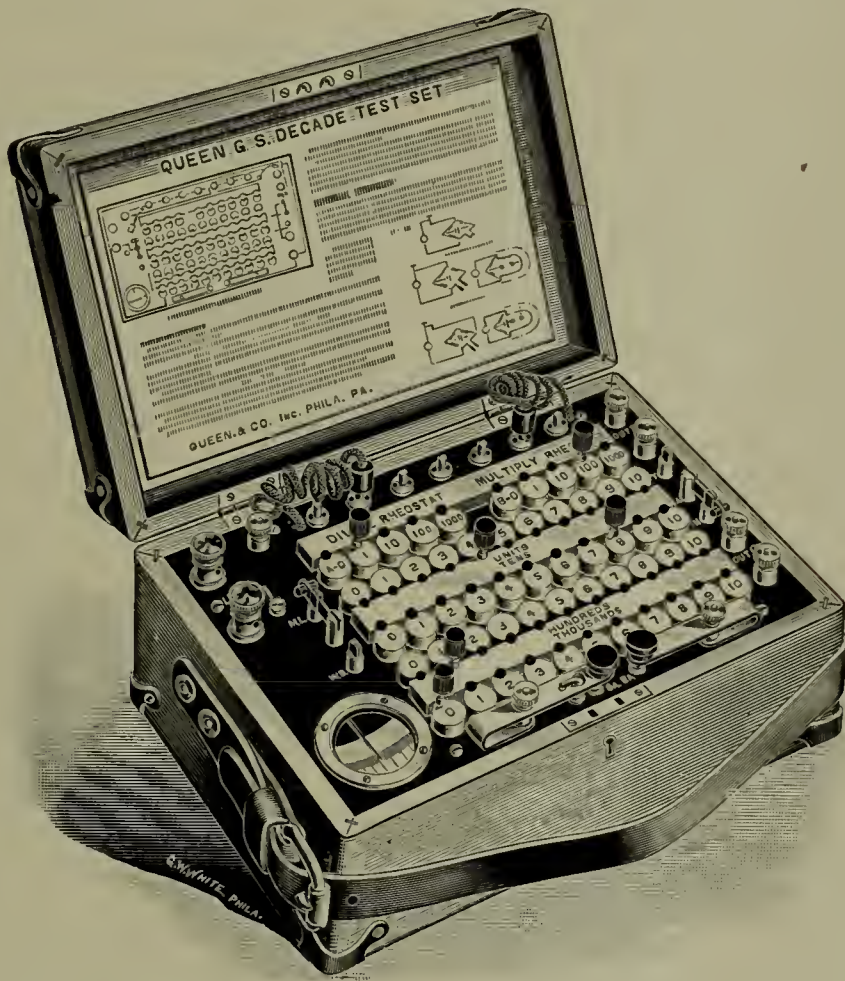
A NEW PORTABLE NAVY DEPARTMENT TESTING SET, MANUFACTURED BY QUEEN & COMPANY, OF PHILADELPHIA
