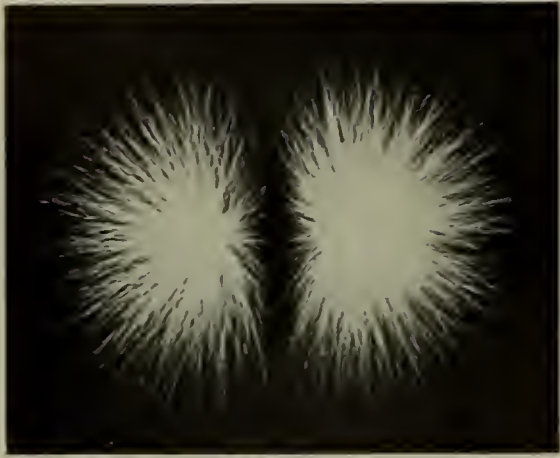
FIG. 5.—A DISCHARGE FROM TWO POLES OF THE SAME SIGN
