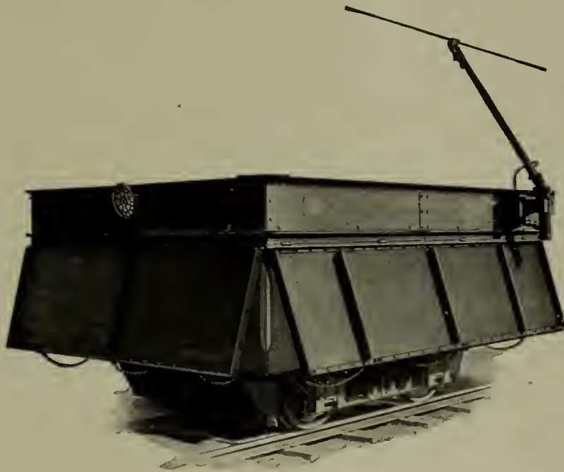
FIG. 2.—ANOTHER VIEW OF THE JEFFREY ELECTRIC DUMP CAR, SHOWING SIDES OPEN
