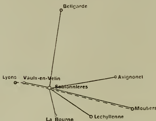
FIG. 1.—DIAGRAM SHOWING RELATIVE LENGTH AND LOCATION OF HIGH-TENSION LINES SUPPLYING HYDRO-ELECTRIC POWER TO LYONS, IN FRANCE
