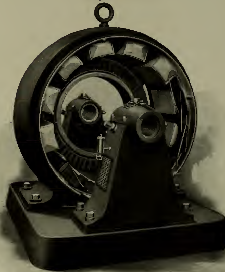
FIGS. 1 AND 2.—INDUCTOR AND ARMATURE OF AN INDUCTOR ALTERNATOR BUILT BY THE WARREN ELECTRIC MANUFACTURING COMPANY, SANDUSKY, OHIO.
