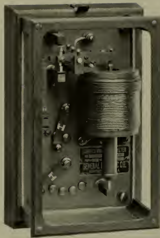
FIG. 10.—POTENTIAL RELAY, OR CONTACT-MAKING VOLTMETER
