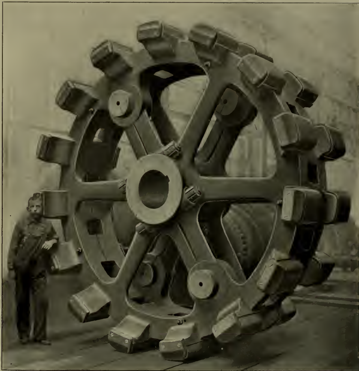
FIG. 6.—INDUCTOR OF A 2000-KW. INDUCTOR ALTERNATOR BUILT BY THE STANLEY-G. I. ELECTRIC MANUFACTURING COMPANY, OF PITTSFIELD, MASS.
