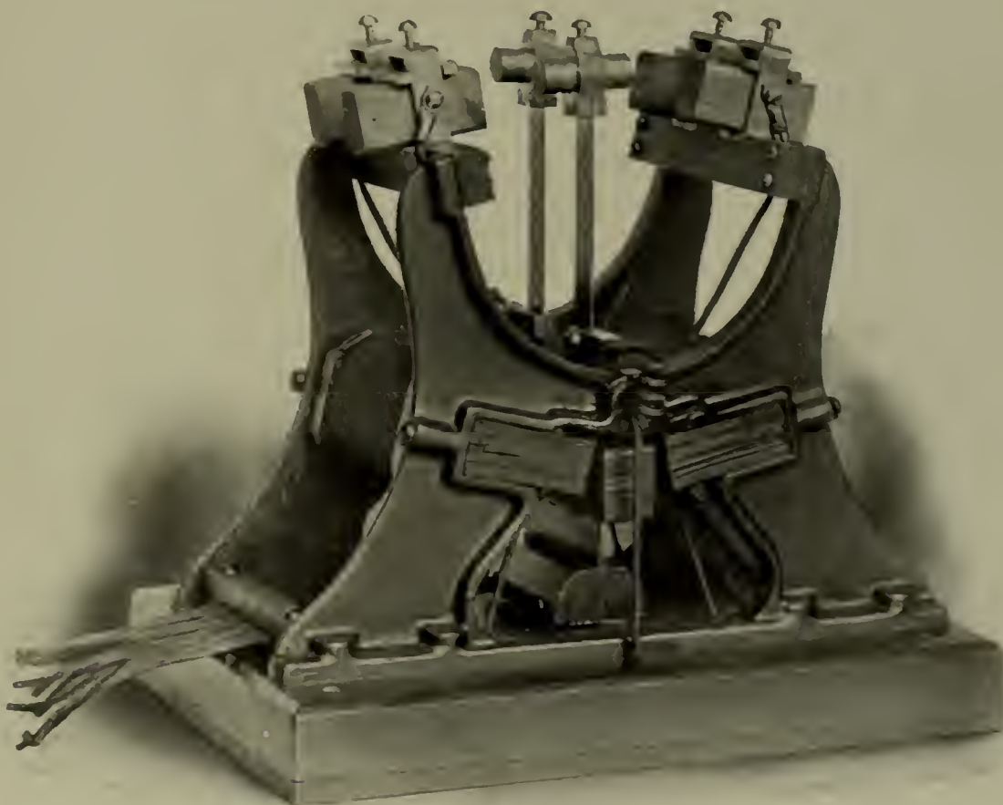
FIG. 16.—REVERSING SWITCH TO REVERSE THE DIRECTION OF THE MOTOR USED ON THE INDUCTION REGULATOR
