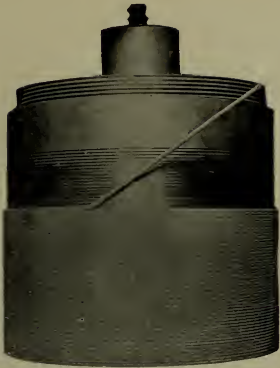
FIG. 13.—UNWINDING COPPER STRIP FOR WIRE
