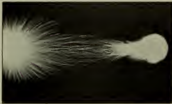
FIG. 6.—A DISCHARGE FROM TWO POLES OF OPPOSITE SIGN
