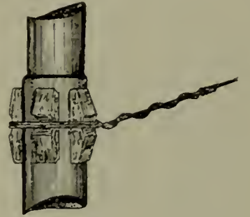
FIG. 9.—TREE BLOCKS FOR PREVENTING INJURY TO THE TREE FROM GUY WIRES
