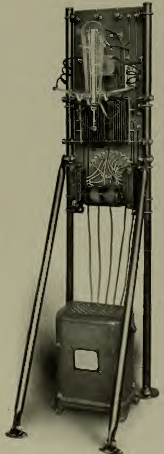
FIG. 2.—REAR VIEW OF THE GENERAL ELECTRIC RECTIFIER OUTFIT IN FIG. 1
