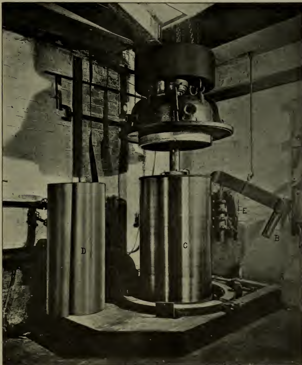
FIG. 8.—PLANT FOR DEPOSITING LARGE COPPER CYLINDERS
