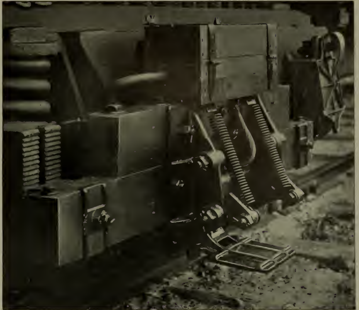
FIG. 4.—INNER POSITION OF THE ADJUSTABLE THIRD-RAIL SHOE
