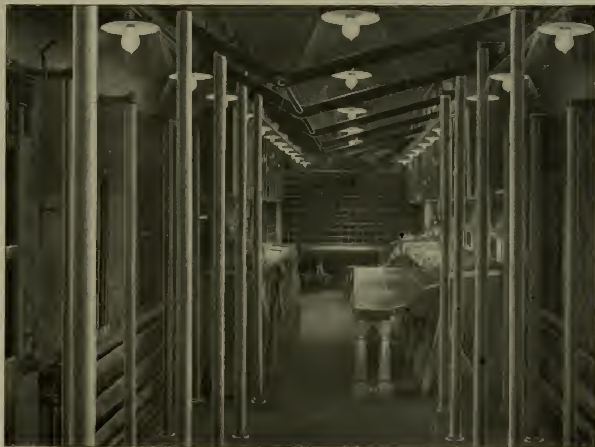
FIG. 19.—A POSTAL CAR LIGHTED ON THE MOSKOWITZ SYSTEM OF THE UNITED STATES LIGHT & HEATING COMPANY
