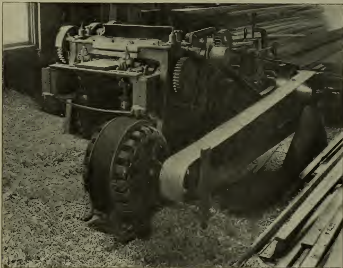
A 15-H. P. WESTINGHOUSE INDUCTION MOTOR DRIVING A PLANER IN THE LUMBER MILL OF THE EGGERS & GRAHAM LUMBER COMPANY, UNIONTOWN, PA.
