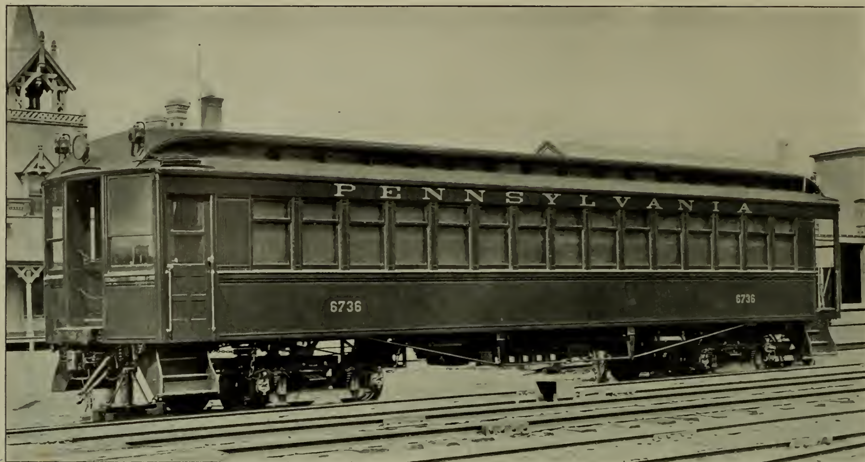
FIG. 9.—A STEEL MOTOR CAR ON THE WEST JERSEY & SEASHORE BRANCH OF THE PENNSYLVANIA RAILROAD
