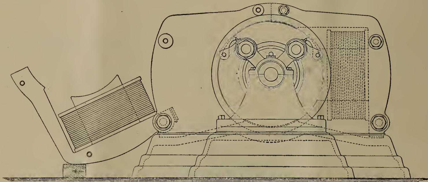
FREEMAN DIRECT CURRENT DYNAMO—REMOVED FIELD COIL.
