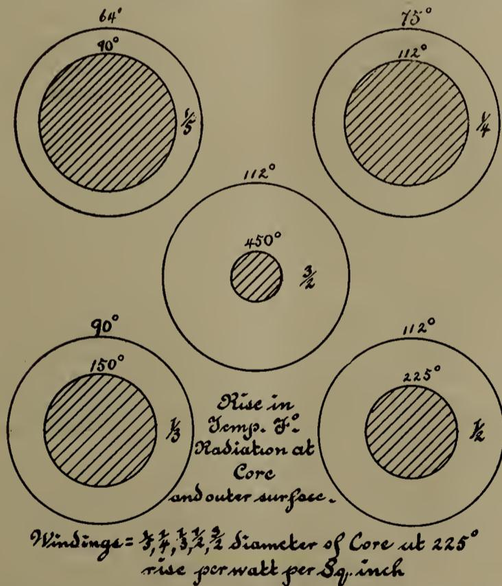
proper coil design, as follows: Determine the watt loss per square inch at core and outer surface by selecting any proportion on the diagram. By this it is inferred that the  $C^2R$  is known; such being the case the dimensions are arrived at by the above system, that is to say, the length of core and depth of winding.
