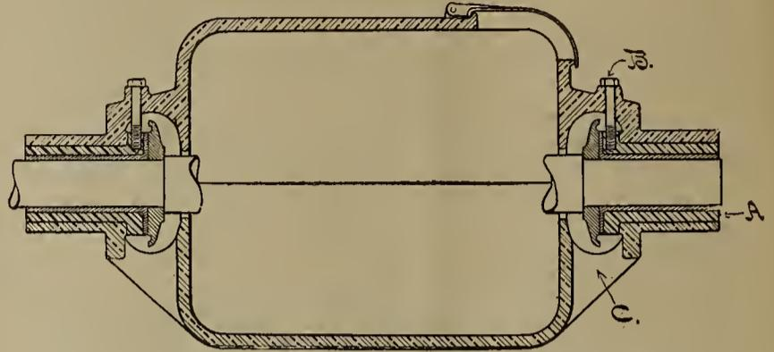
FIG. 2.—SECTIONAL VIEW OF MOTOR CASING AND BEARINGS.
