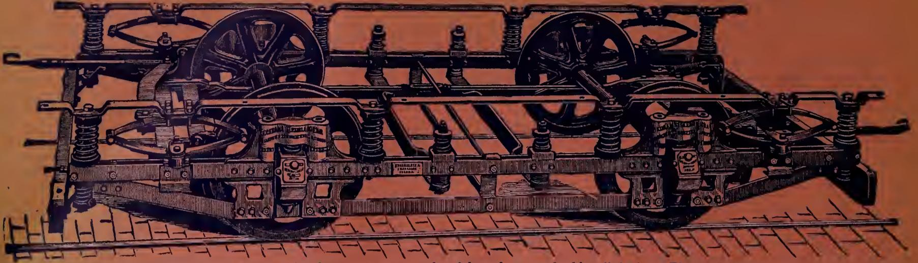
Constructed with hot rivets; all parts machine fitted and guaranteed. Adopted as standard by all the large Electric Railways in Brooklyn, New York, and Jersey City. Cost of maintenance guaranteed to be less than any other truck. For pricelist, descriptive catalogue and blue prints, apply to
