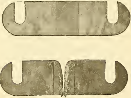
Fuse Intact and Fuse Blown.
