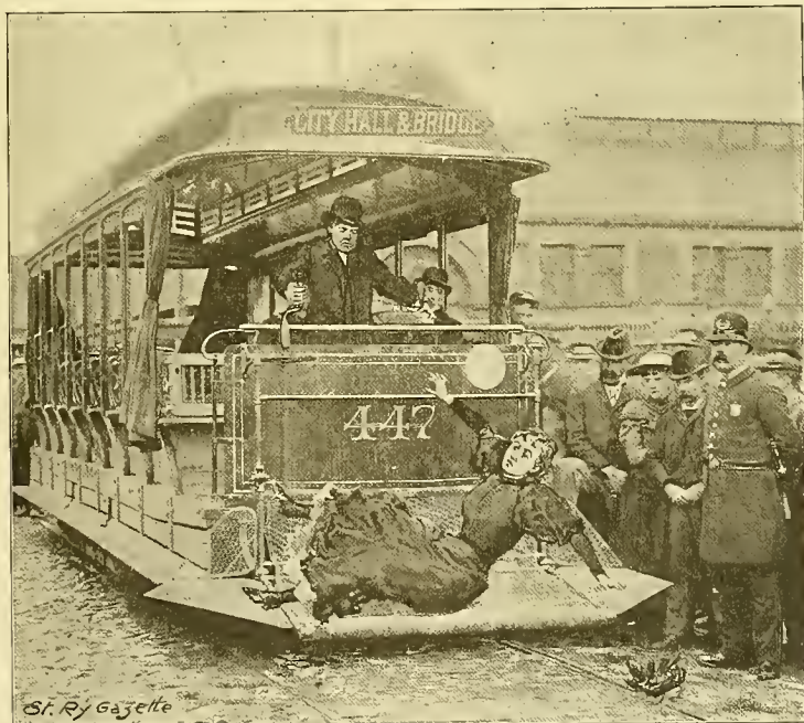
FIG. 4.—HOW THE FENDER COLLAPSES AND PICKS UP THE PEDESTRIAN.
