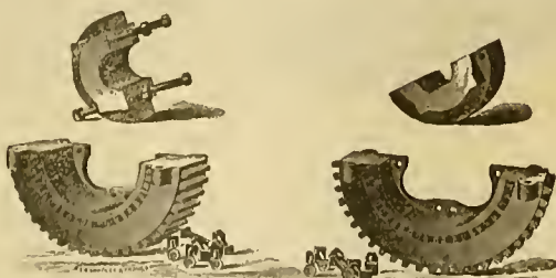
FIG. 4.—ELECTRIC RAILWAY GEARING—CONSTRUCTION OF SPLIT GEAR—WOODEN TEETH.
