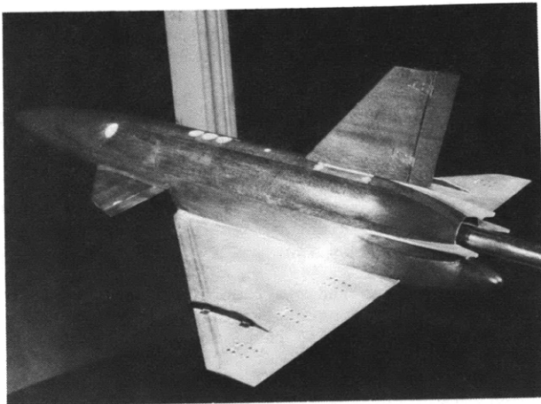
Figure 4 - NSRDC VATOL RPV Wind Tunnel Model (30% Scale)
