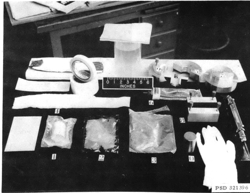
Figure A21 – Various Items Used in Testing Specimens after Exposure to Artificial Sea Water
