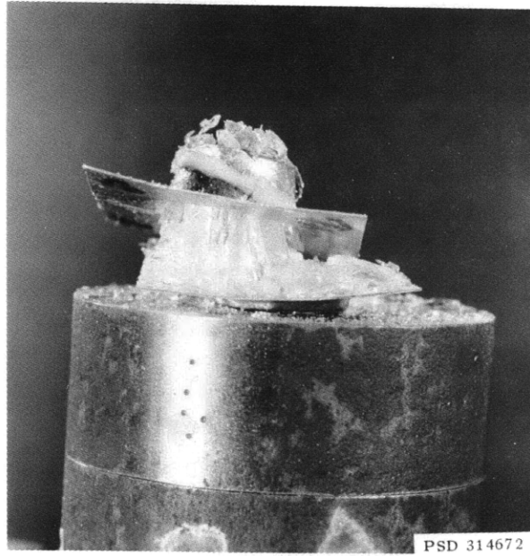
Figure A11c – Broken Specimens after Removal of Upper Bearing Block
