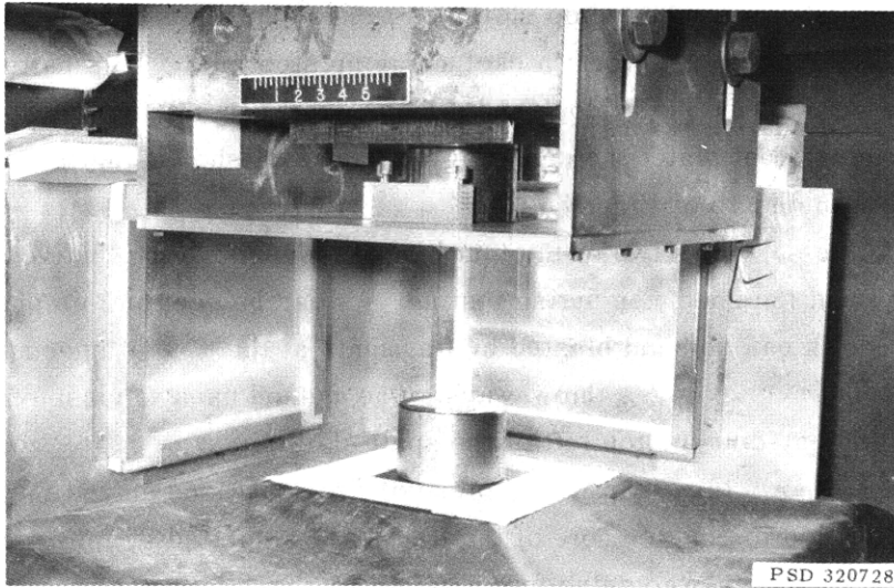
Figure A16 – Rubber Drop Cloth Used in Test Setup to Protect Swivel Head and Showing Part of Spall Shield
