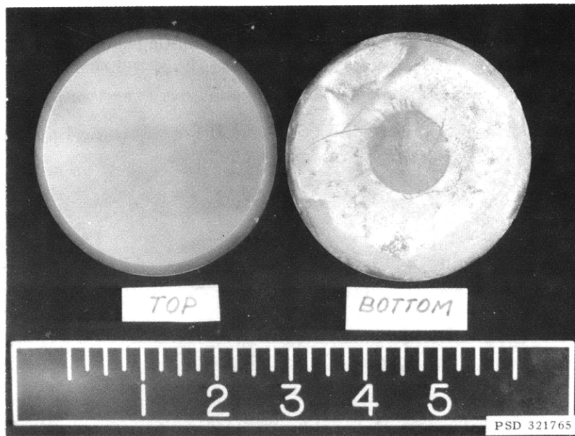
Figure A28c – Bearing Blocks after Test
