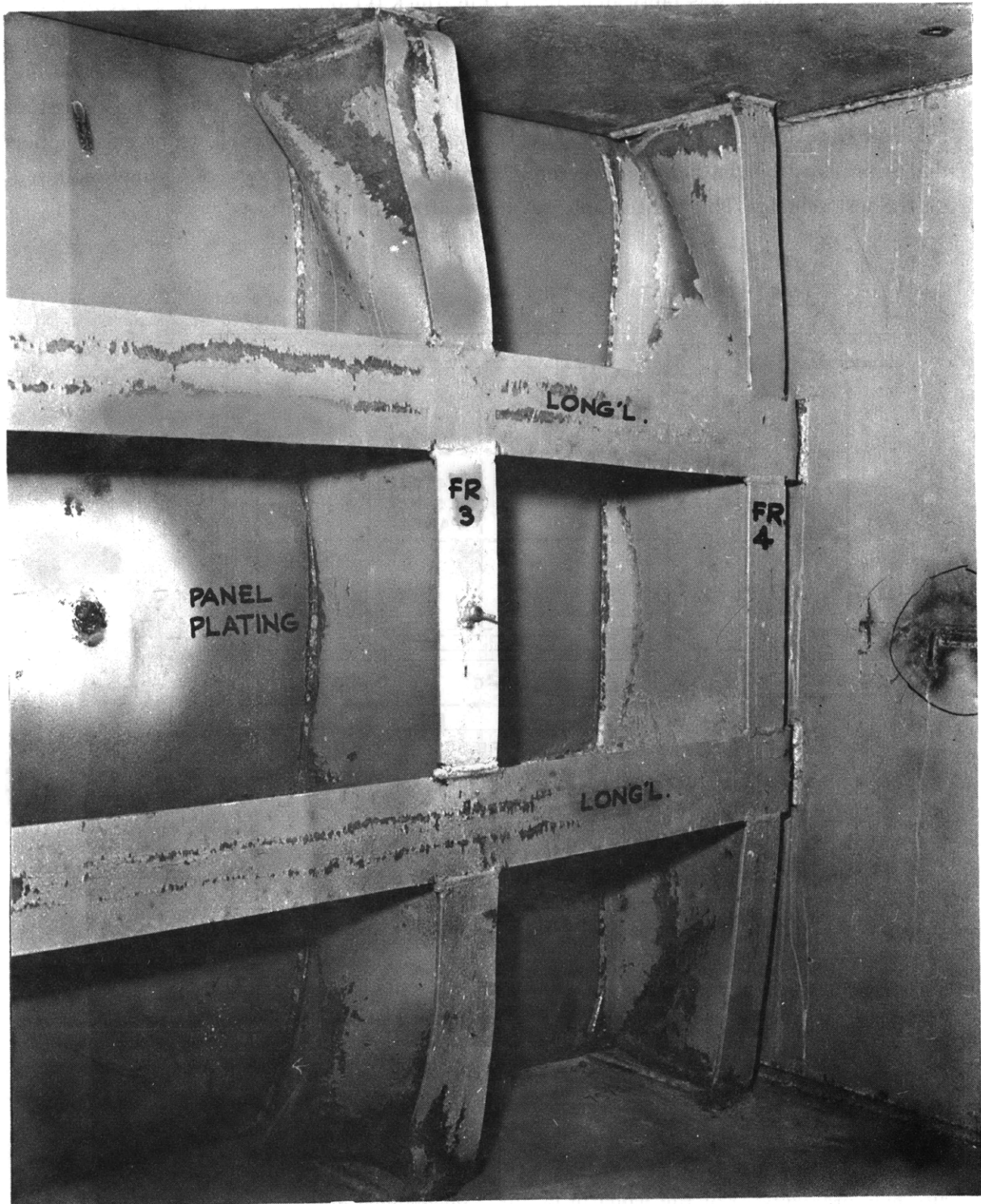
Figure 2 - Test Panel Showing Frames and Longitudinals
