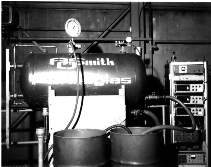
Figure 8a - Head Tank and Associate Instrumentation
