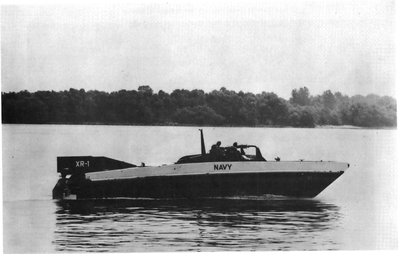
Figure 2 - CAB XR-1 Experimental Research Craft at a Speed of 30 Knots
