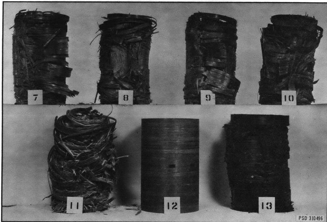
Figure 4 - Cylinders B-7 to B-13 after Failure
