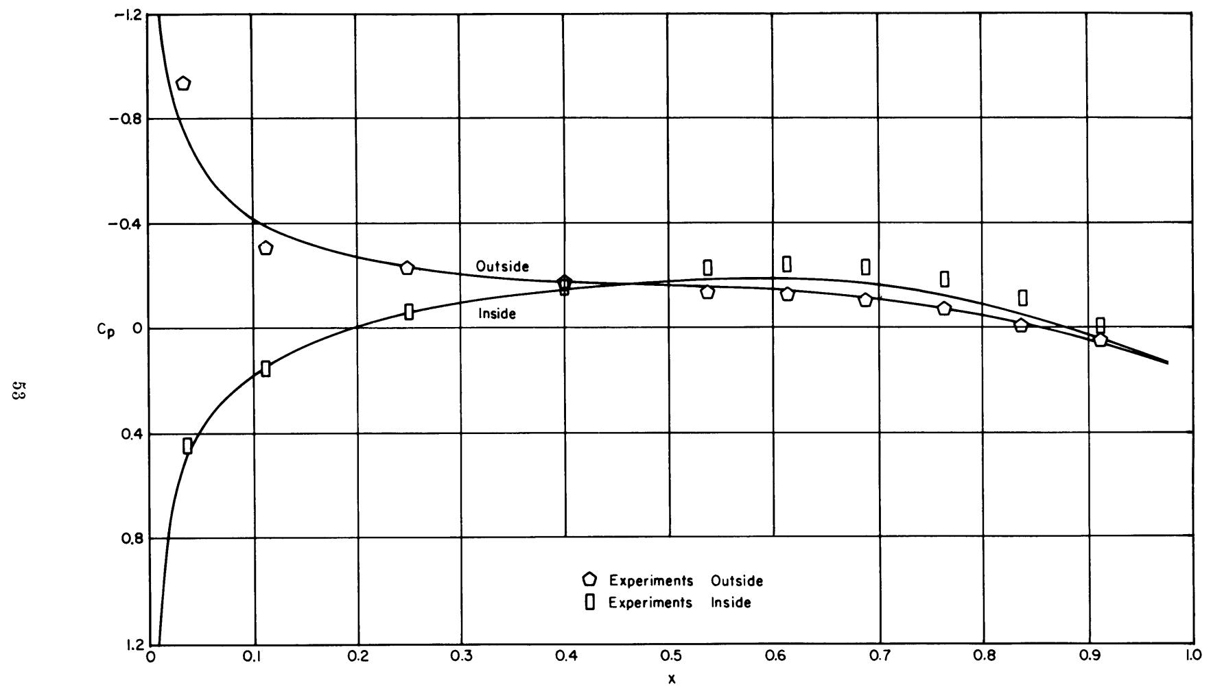
Figure 18 - Pressure Distribution for BTZ Duct,  $\alpha_r = 9$  Degrees and  $\phi = 0$  Degrees
