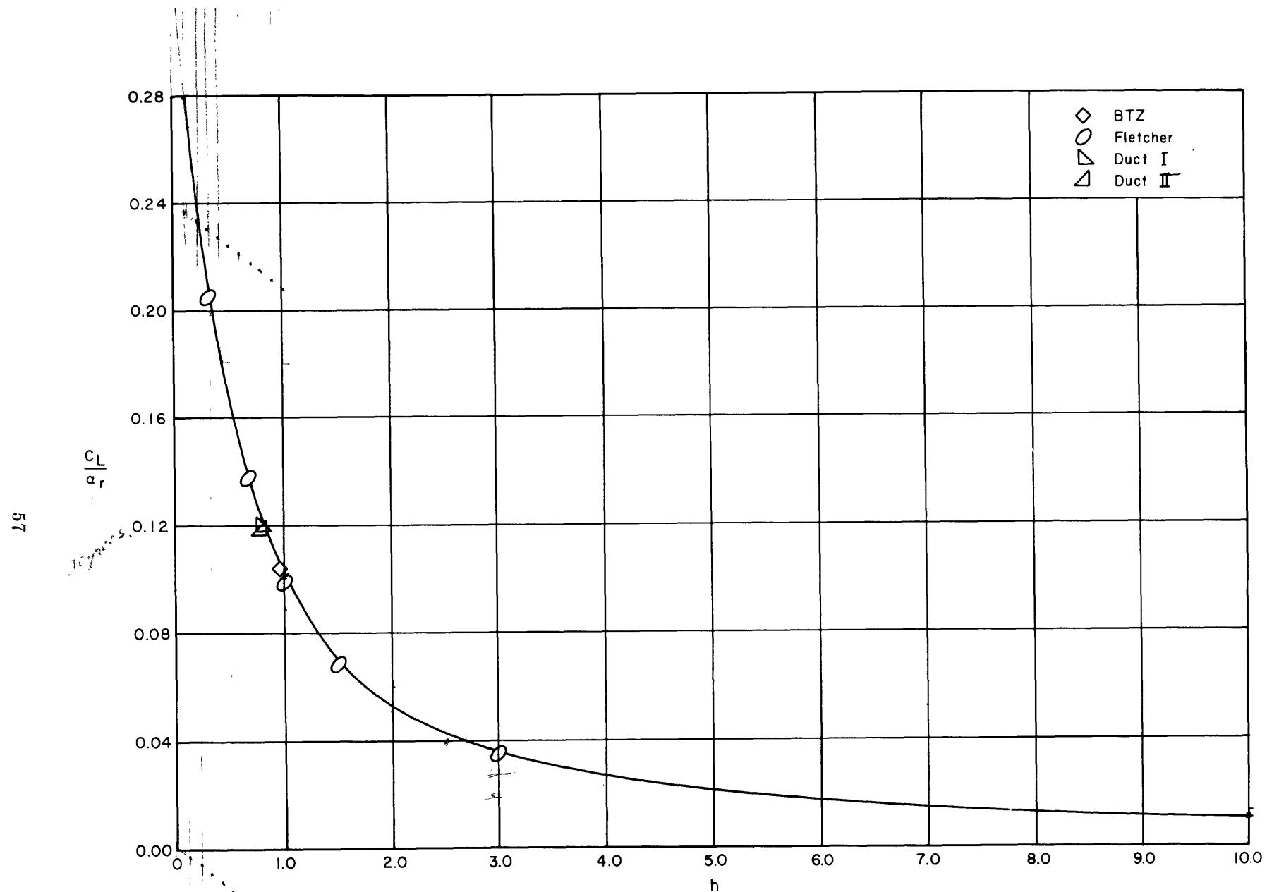
Figure 22 - Lift Curve Slope as Function of Chord-Diameter Ratio
