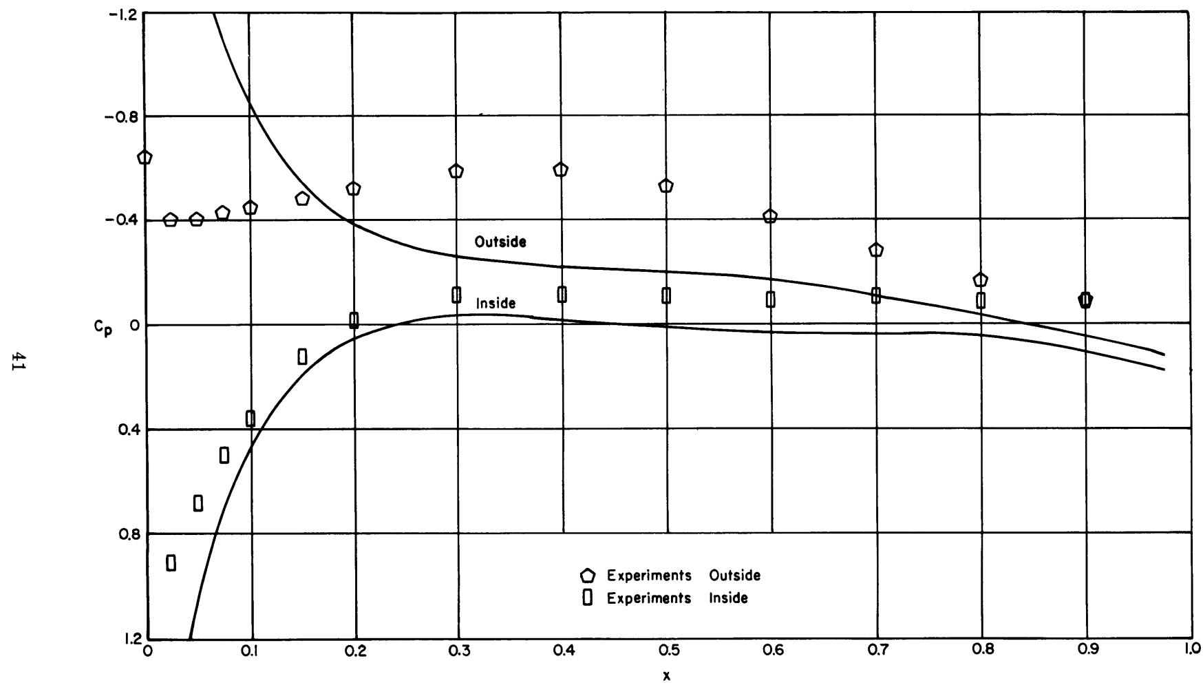
Figure 6 - Pressure Distribution for Duct I,  $\alpha_r = 6$  Degrees and  $\phi = 0$  Degrees
