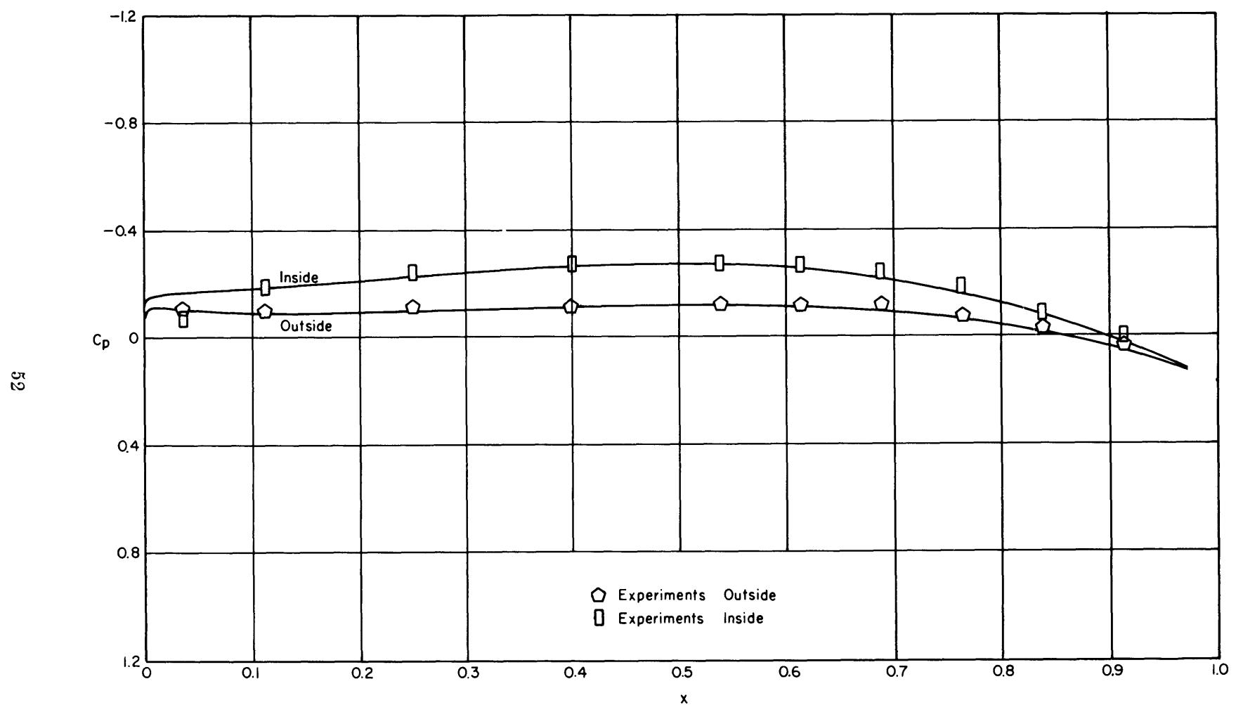
Figure 17 - Pressure Distribution for BTZ Duct at Zero Angle of Attack ( $\alpha_r = 0$ )
