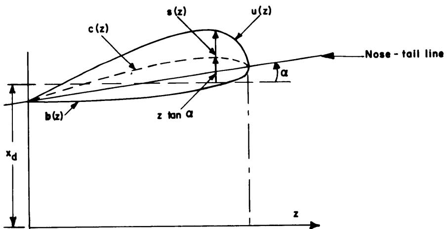
Figure 2 - Delineation of the Annular Airfoil Section
