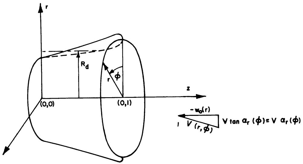
Figure 1 - The Annular Airfoil Coordinate System
