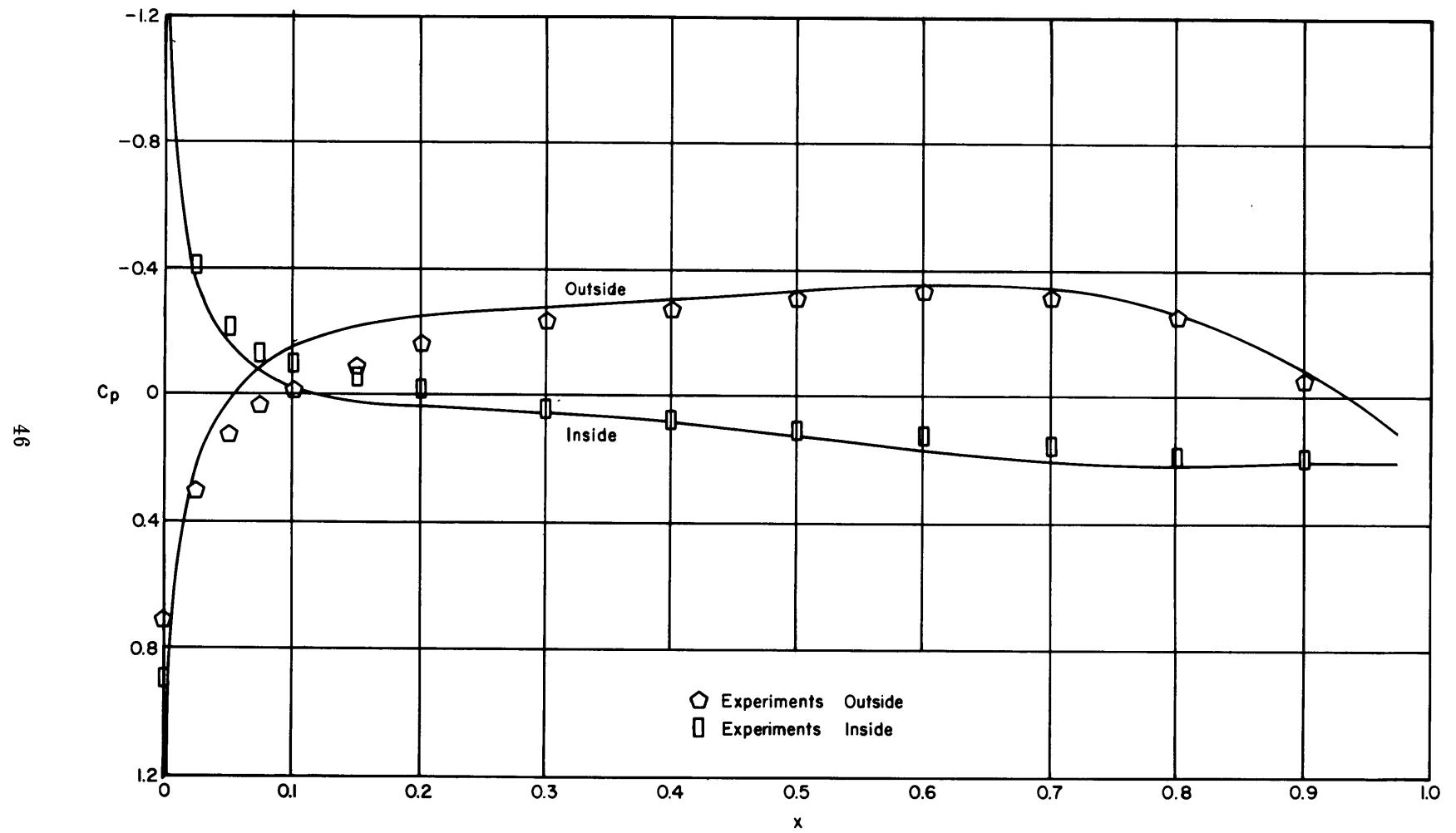
Figure 11 - Pressure Distribution for Duct II,  $\alpha_r = 4$  Degrees and  $\phi = 180$  Degrees
