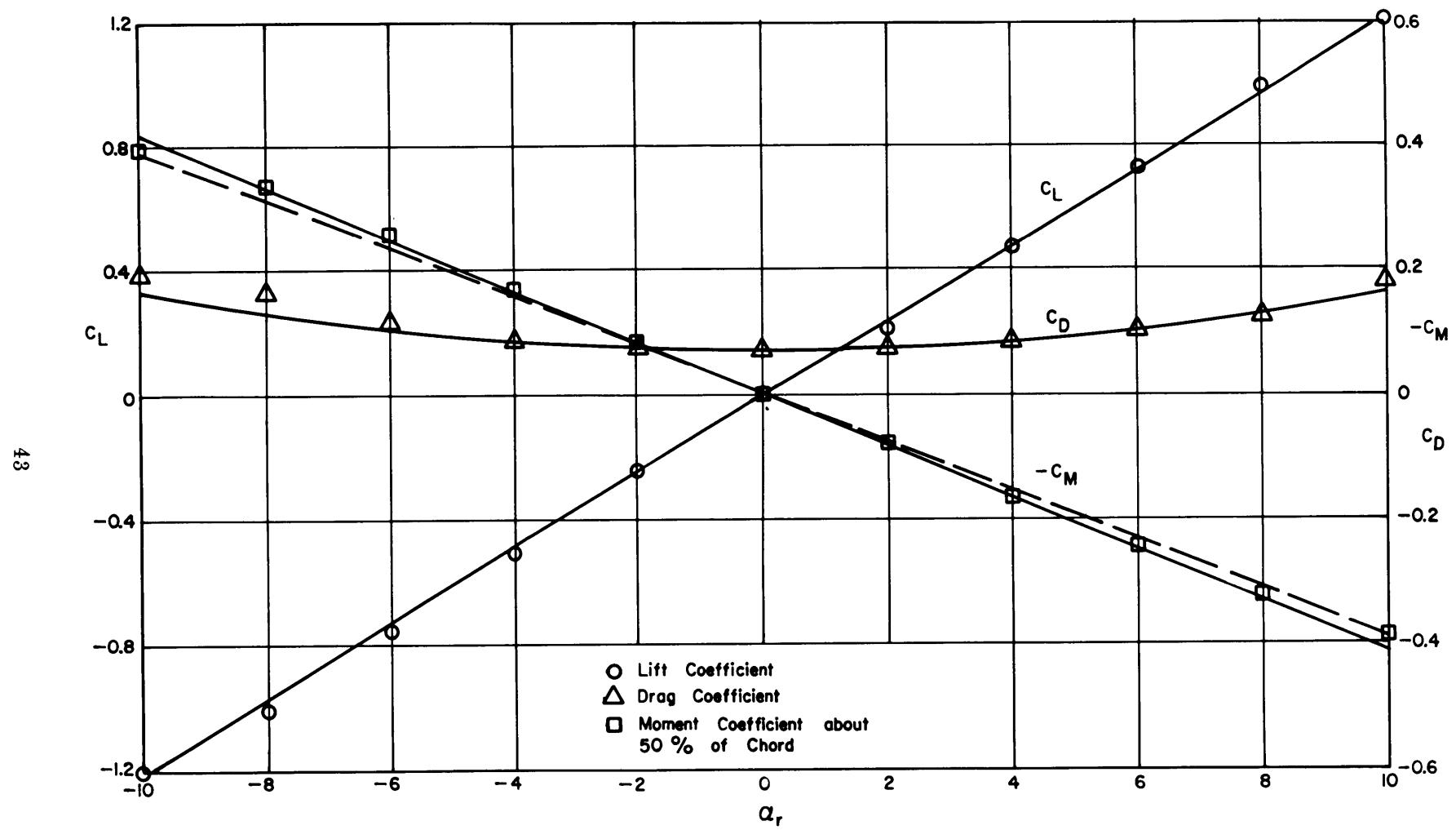
Figure 8 - Lift, Drag, and Moment Coefficients for Duct II
