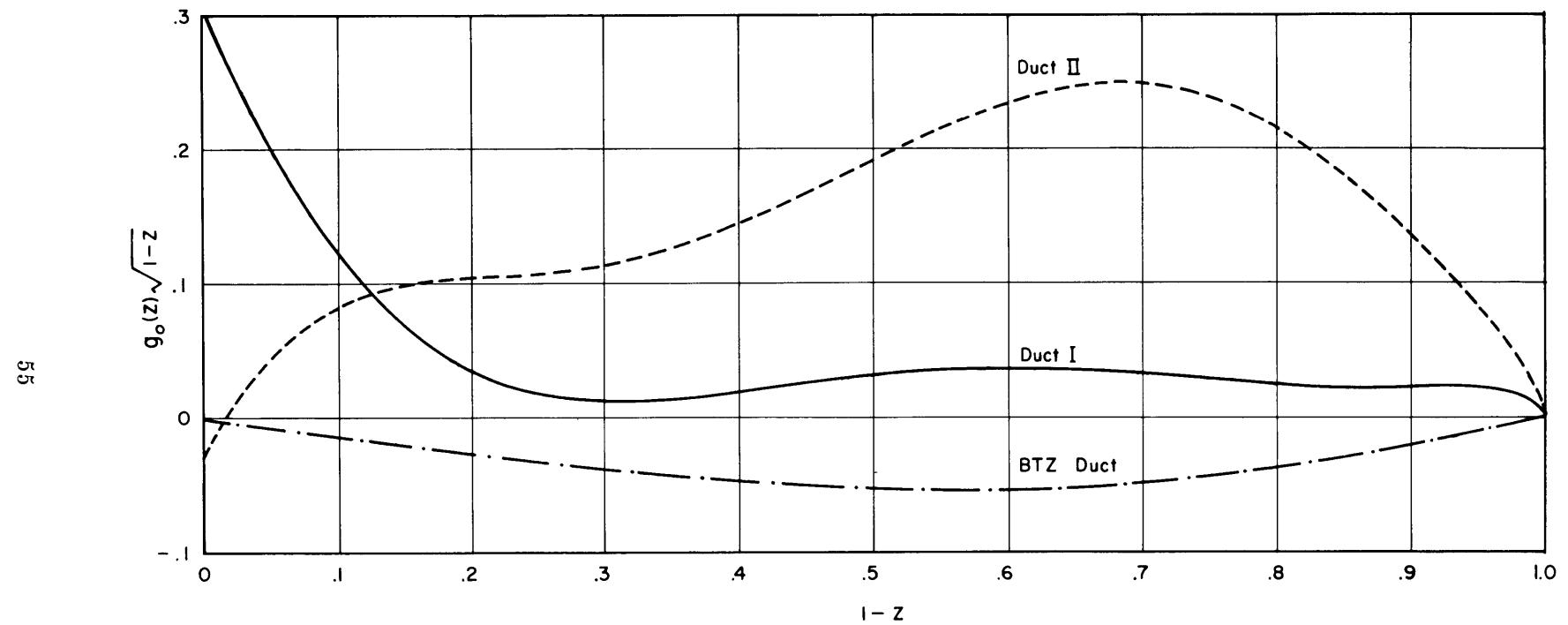
Figure 20 - Circulation Distribution for the Three Ducts
