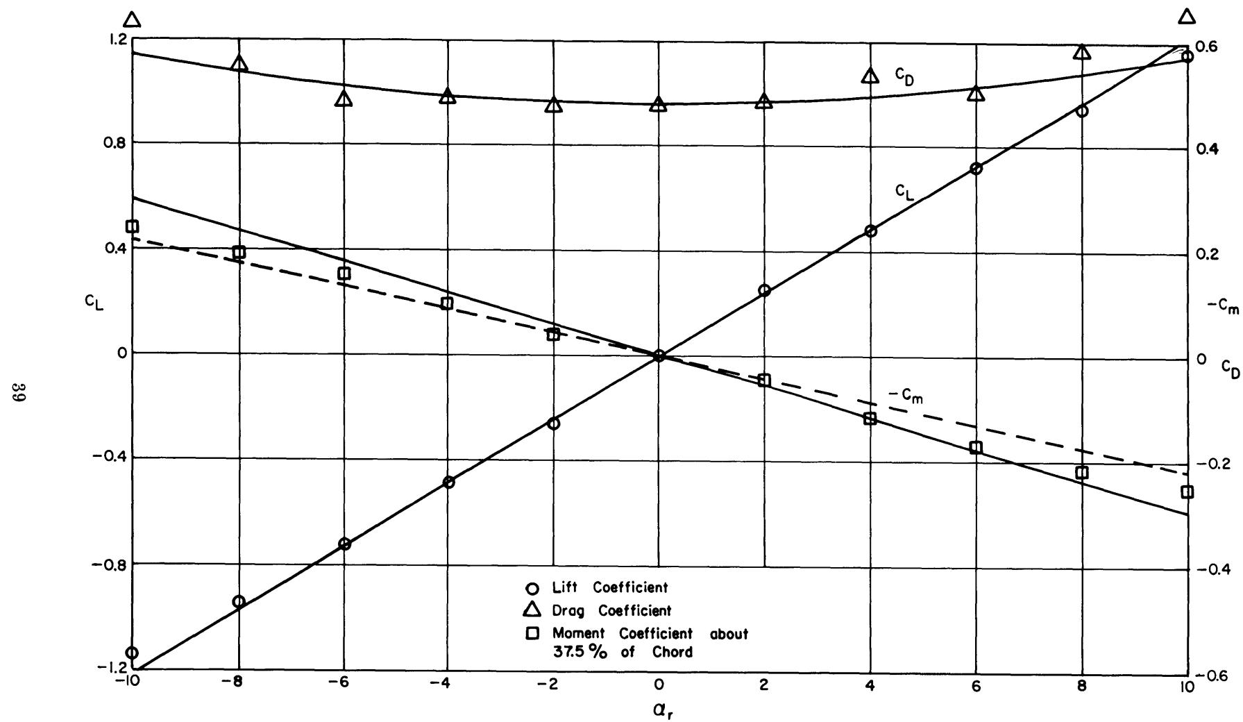
Figure 4 - Lift, Drag, and Moment Coefficients for Duct I
