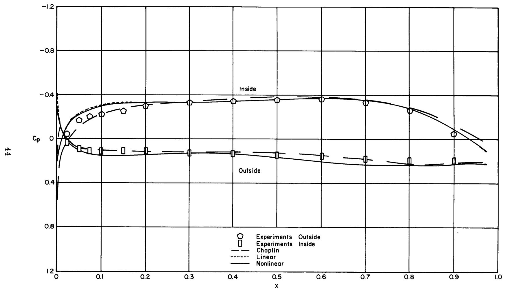
Figure 9 - Pressure Distribution for Duct II at Zero Angle of Attack ( $\alpha_r = 0$ )
