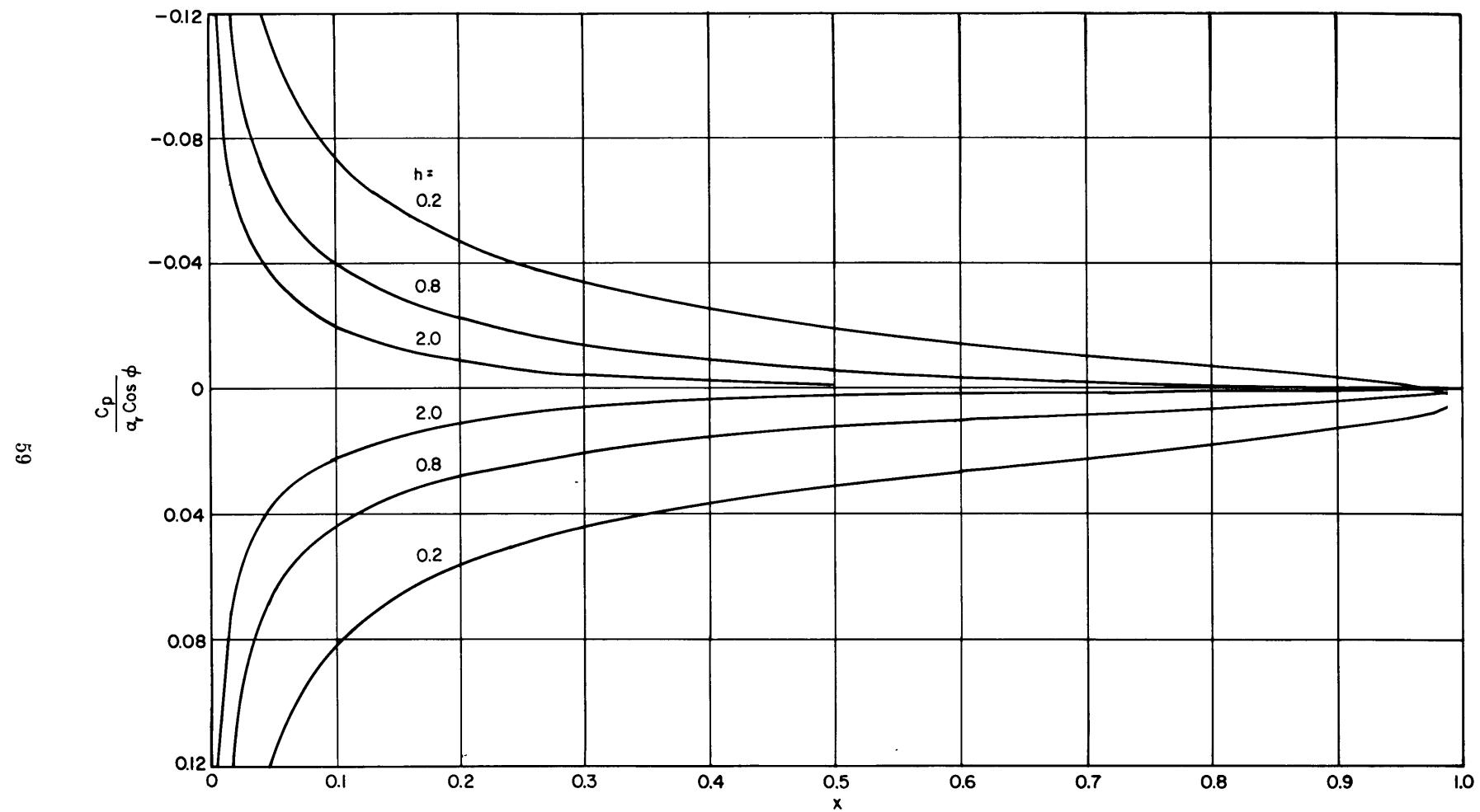
Figure 24 - Pressure Distribution as a Function of Duct Angle of Attack and Chord-Diameter Ratio
