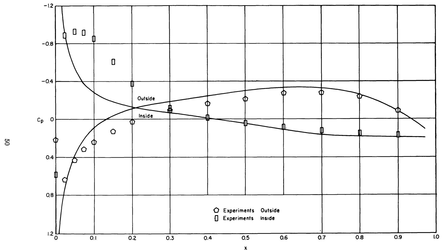
Figure 15 - Pressure Distribution for Duct II,  $\alpha_r = 10$  Degrees and  $\phi = 180$  Degrees
