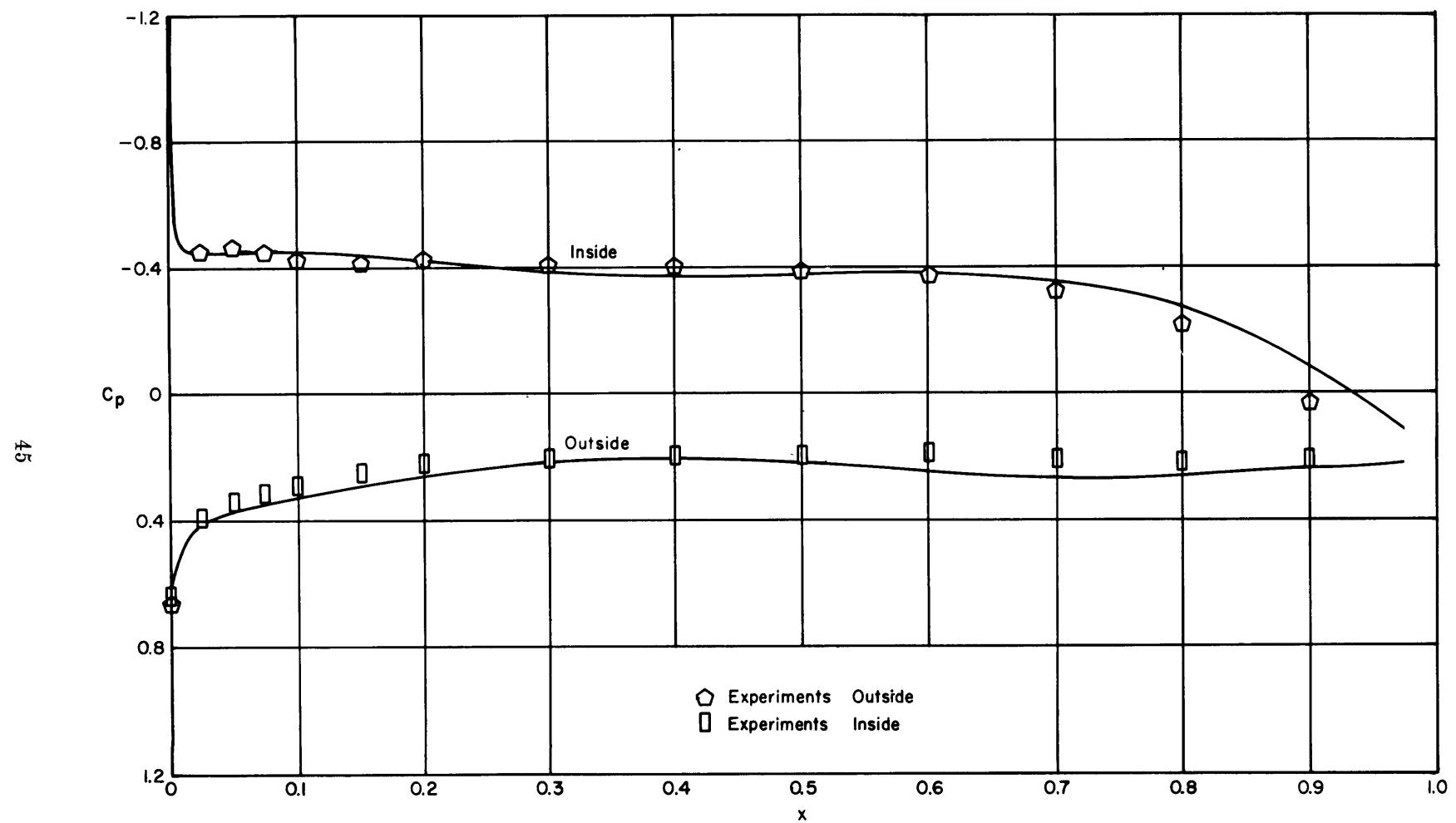
Figure 10 - Pressure Distribution for Duct II,  $\alpha_r = 4$  Degrees and  $\phi = 0$  Degrees
