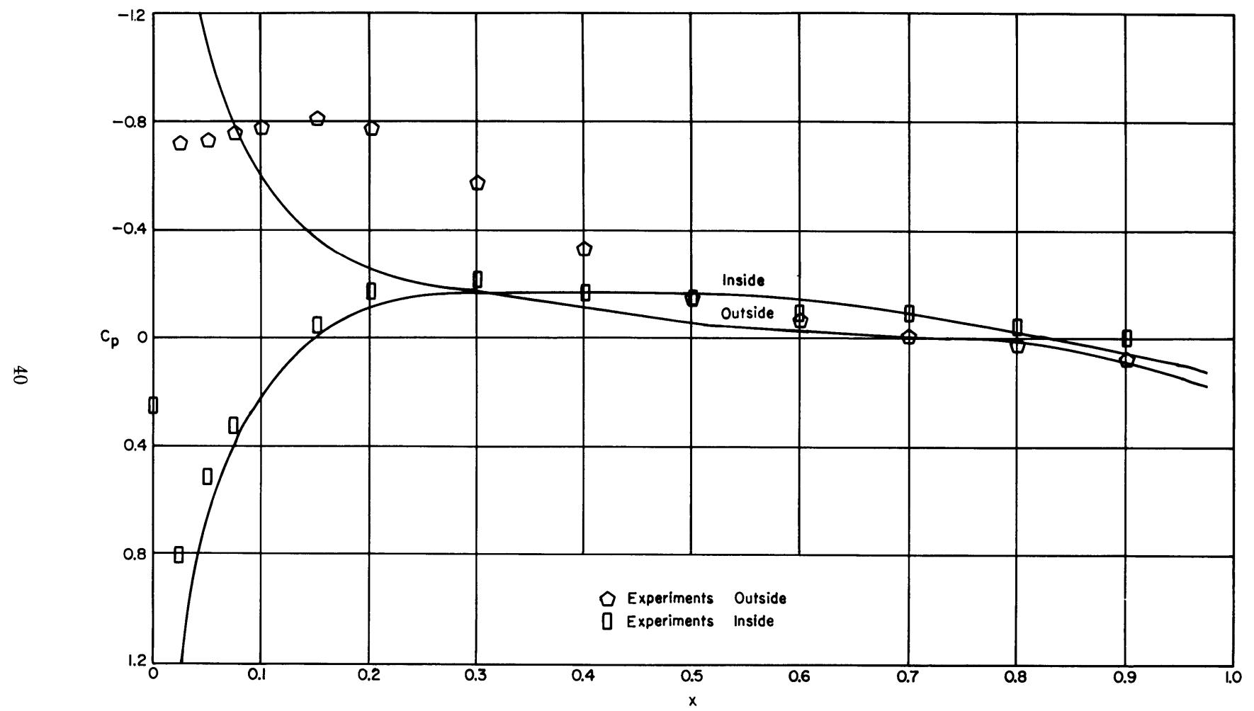
Figure 5 - Pressure Distribution for Duct I at Zero Angle of Attack ( $\alpha_r = 0$ )
