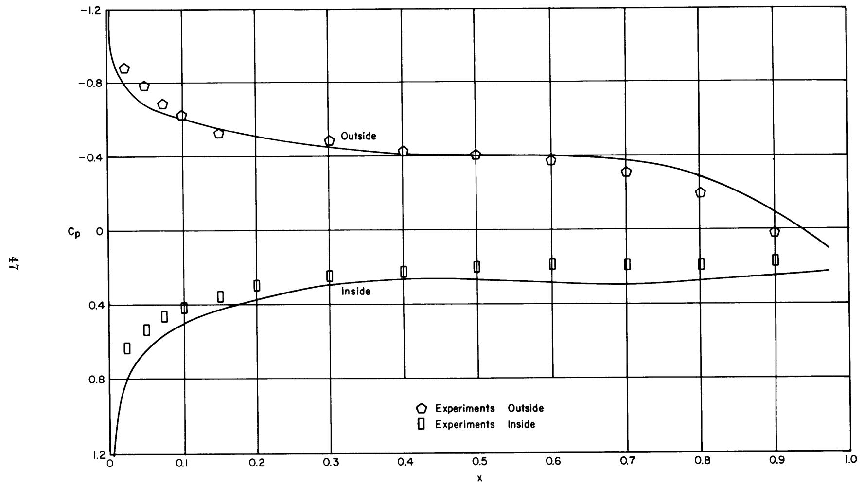
Figure 12 - Pressure Distribution for Duct II,  $\alpha_r = 8$  Degrees and  $\phi = 0$  Degrees
