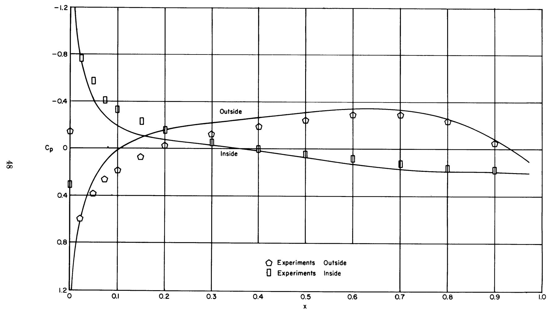
Figure 13 - Pressure Distribution for Duct II,  $\alpha_r = 8$  Degrees and  $\phi = 180$  Degrees
