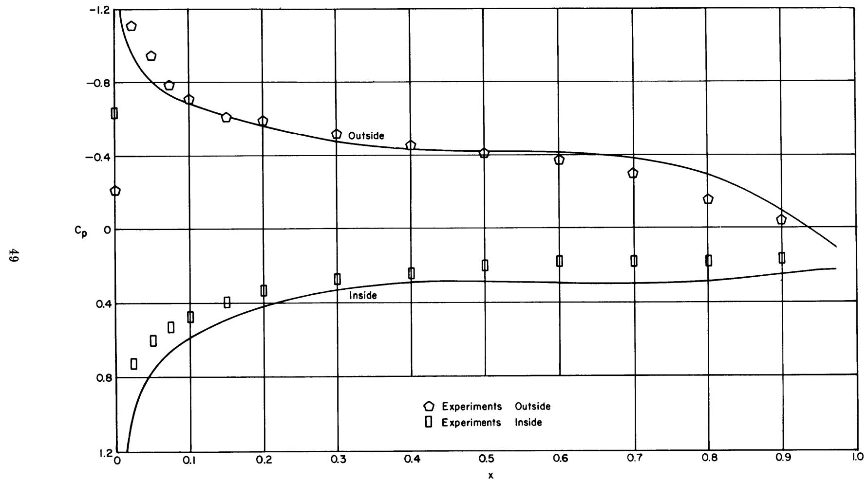
Figure 14 - Pressure Distribution for Duct II,  $\alpha_r = 10$  Degrees and  $\phi = 0$  Degrees
