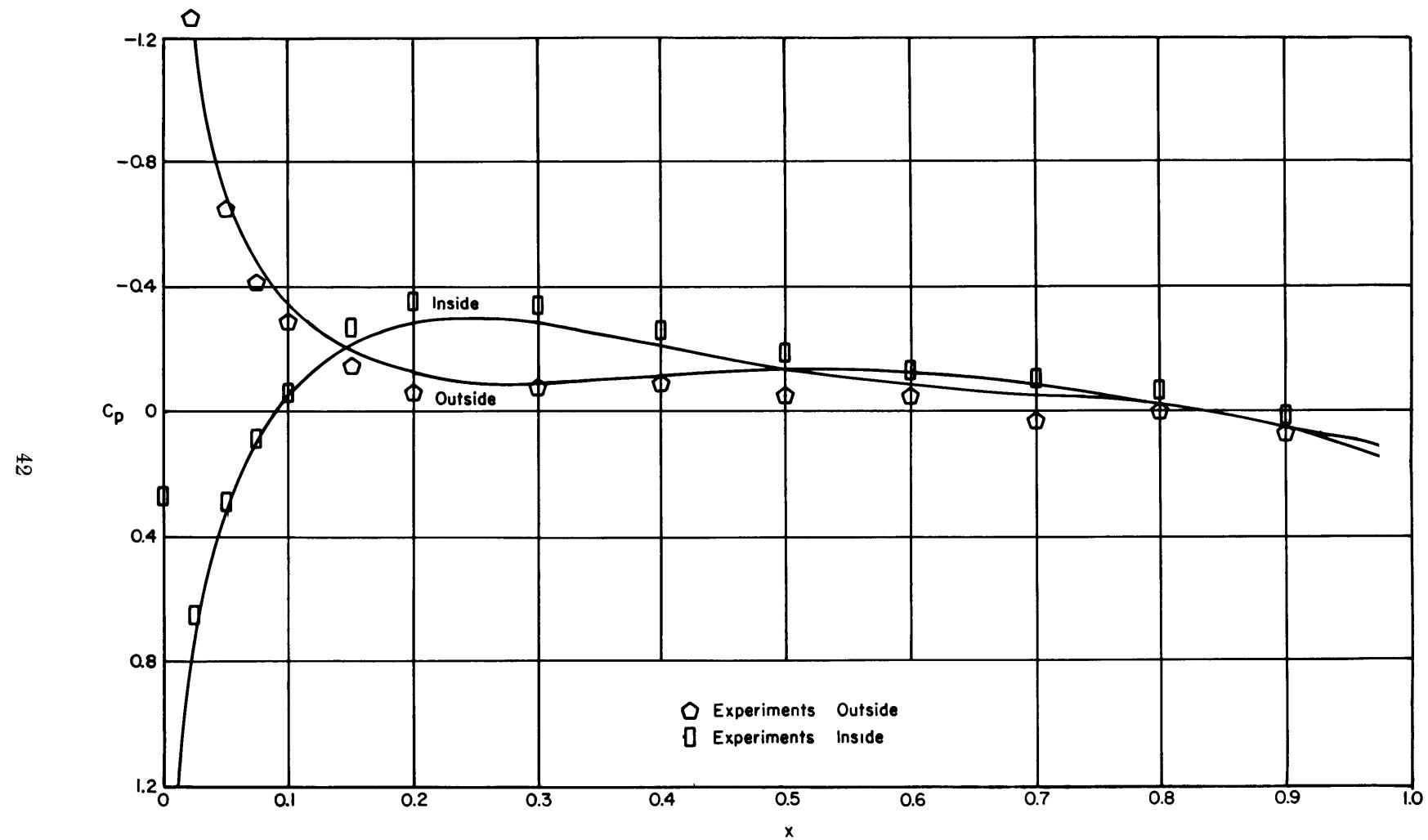
Figure 7 - Pressure Distribution for Duct I,  $\alpha_r = 6$  Degrees and  $\phi = 180$  Degrees
