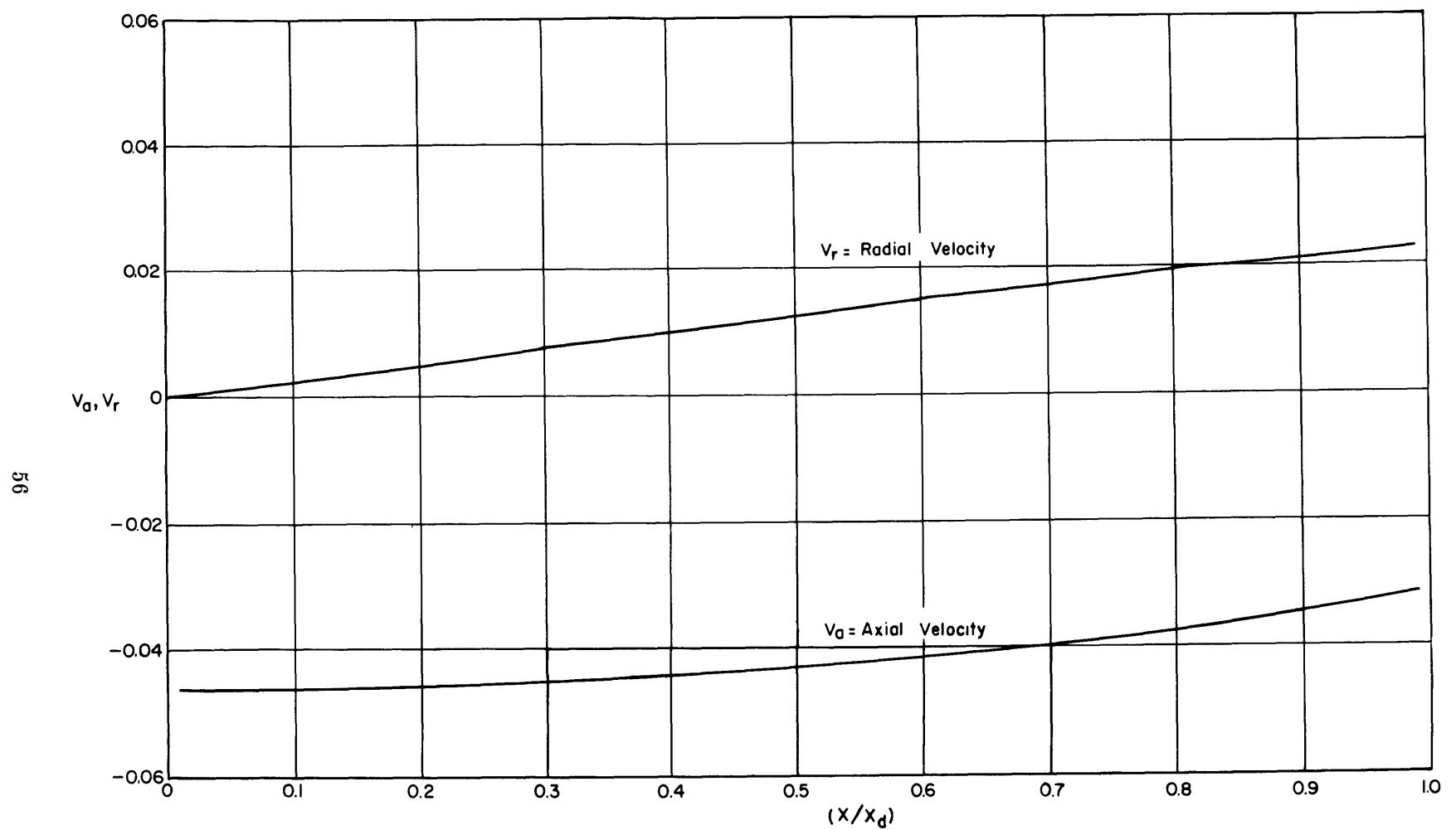
Figure 21 - Radial Variation of Velocity at  $\frac{1}{2}$  Chord Point for Duct II
