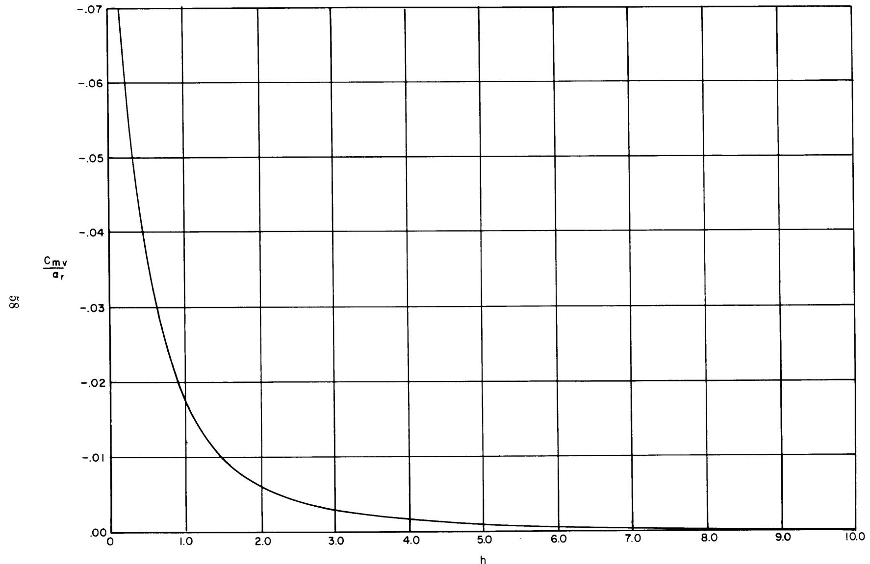
Figure 23 - Moment from Vertical Forces as Function of Duct Angle of Attack and Chord-Diameter Ratio
