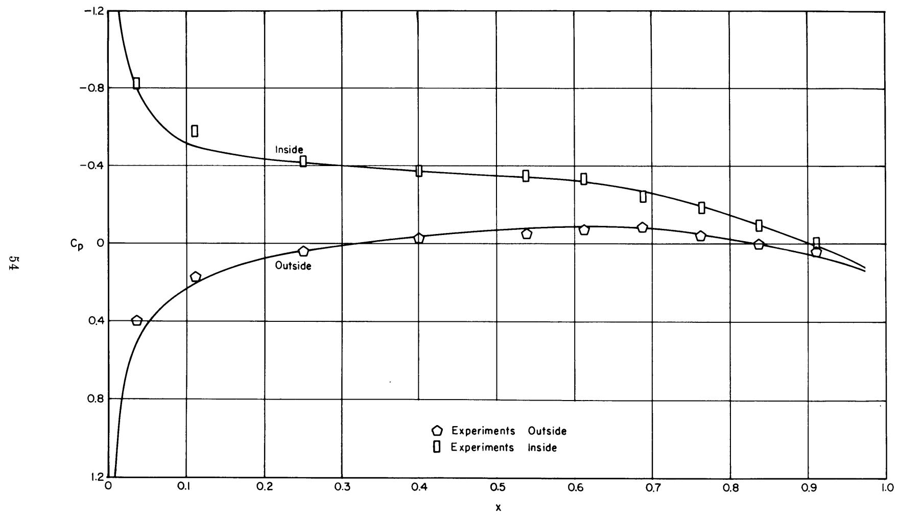
Figure 19 - Pressure Distribution for BTZ Duct,  $\alpha_r = 9$  Degrees and  $\phi = 180$  Degrees
