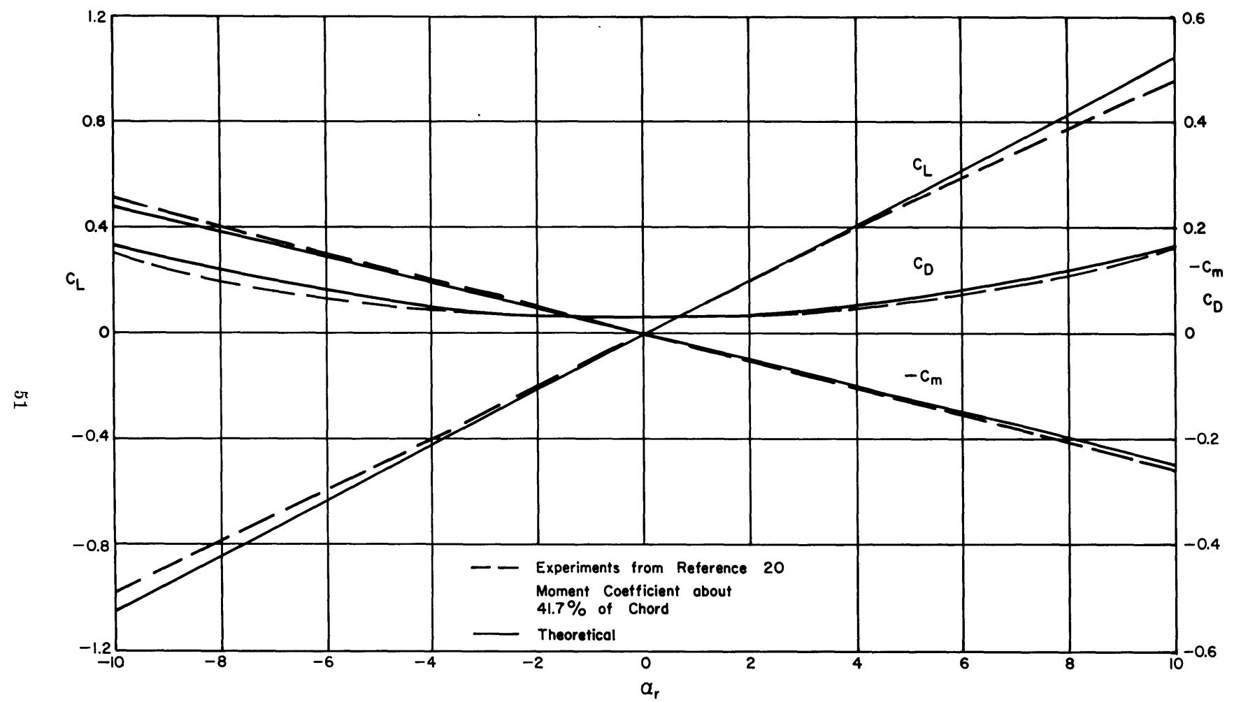
Figure 16 - Lift, Drag, and Moment Coefficients for BTZ Duct
