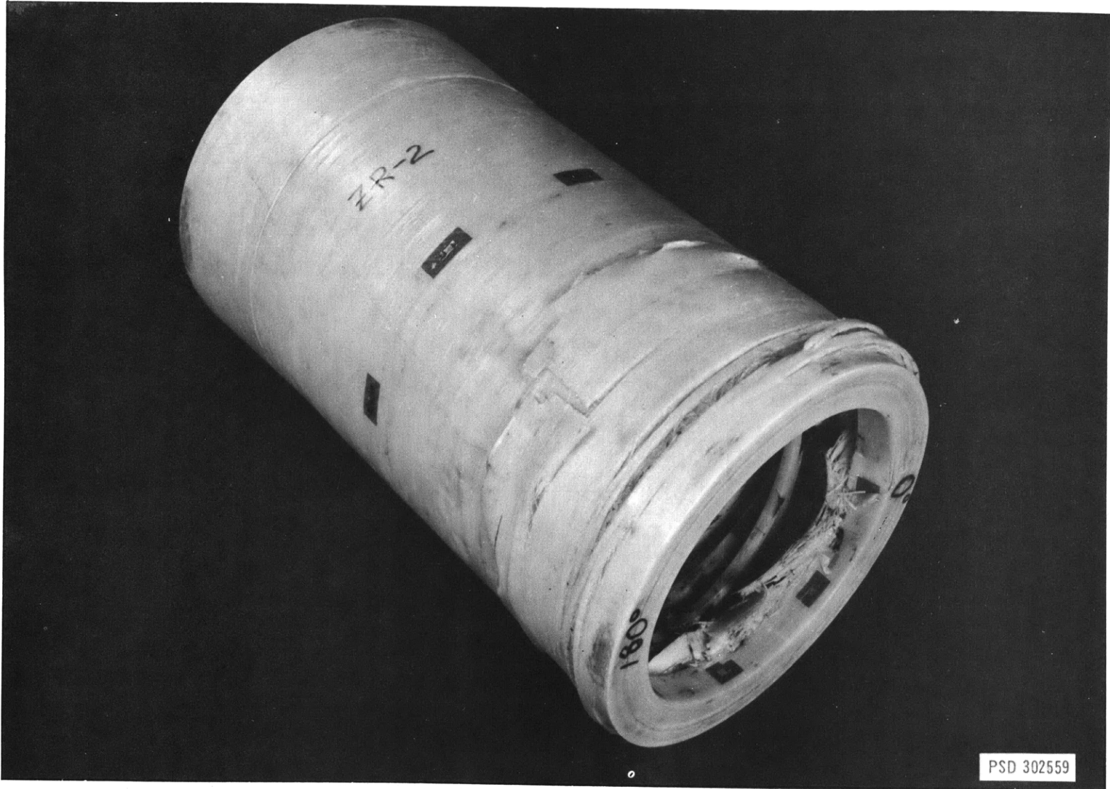
Figure 16 - End View of Model ZR-2 after Failure
