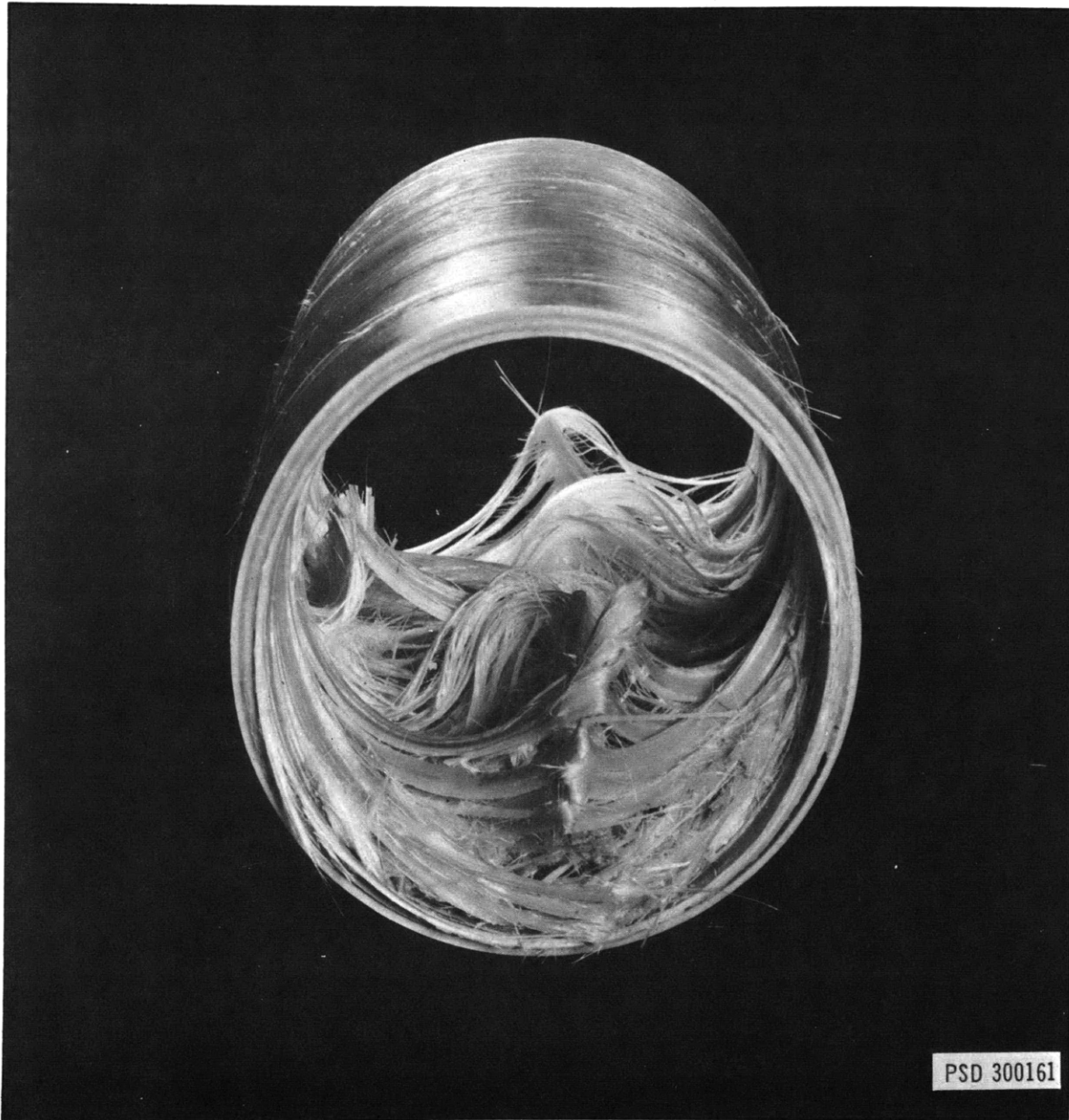
Figure 8 - Interior View of Model B-1 after Failure
