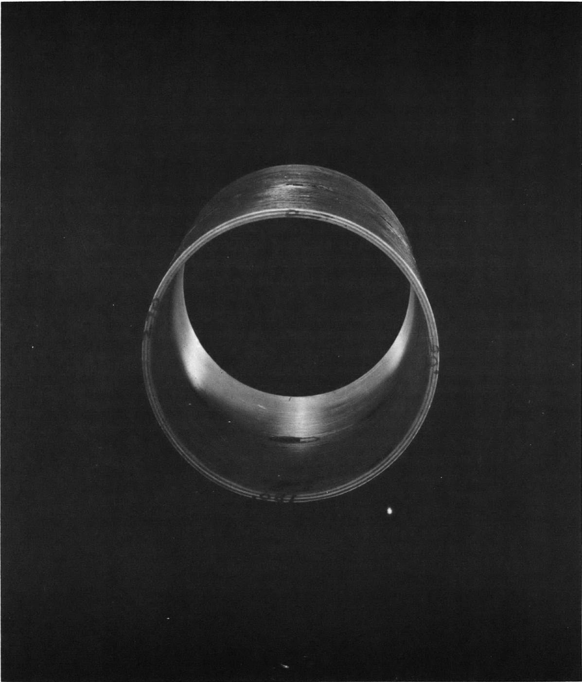
Figure 12 - End View of Model B-3 after Failure
