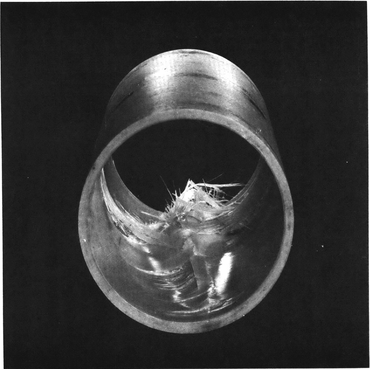
Figure 7 - Interior View of Model Z-1 after Failure
