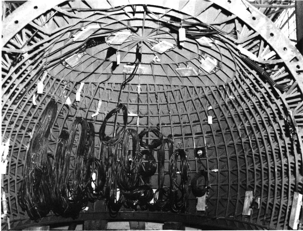
Figure 2 – Interior View of Removable Section of Bow Dome
