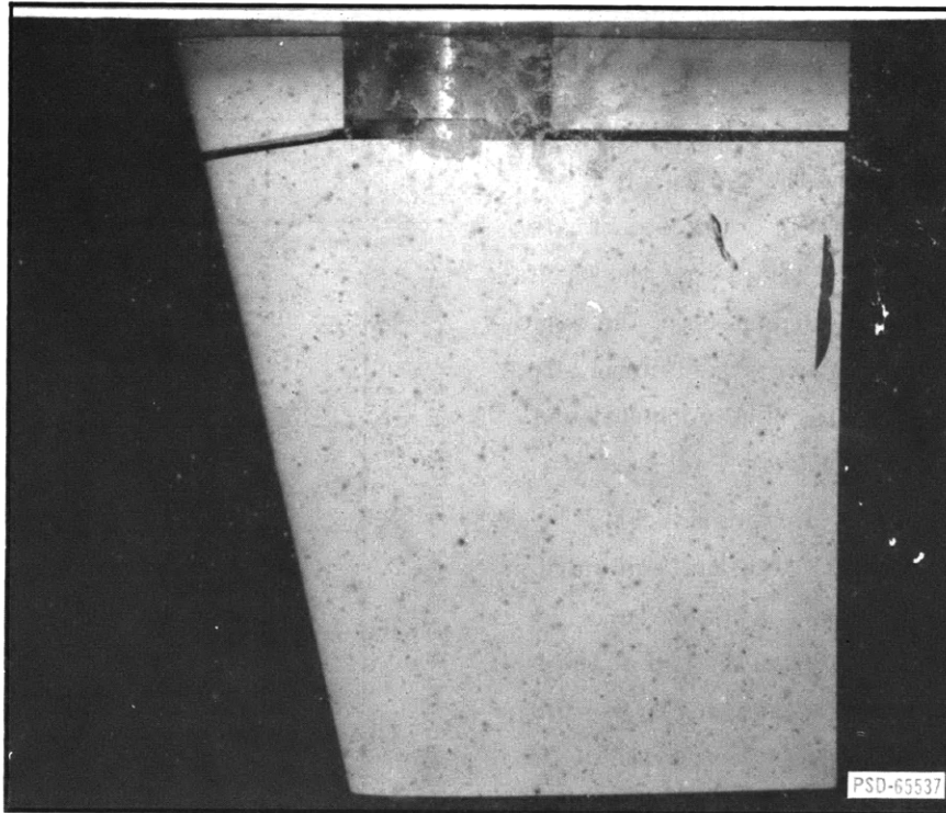
Figure 10 – Cavitation on Model Rudders at 0 Degree, 34 Knots
