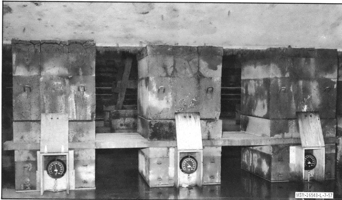
Figure 16 - View of Instrumented Keel Blocks under USS BENNINGTON (CVS 20)
