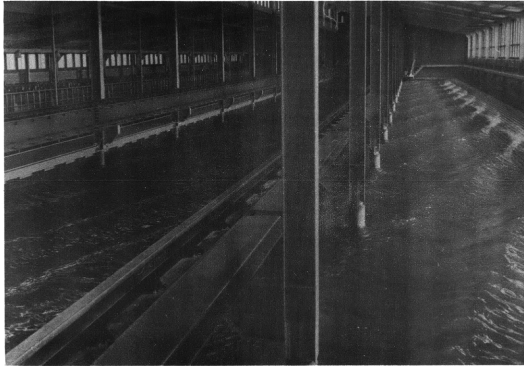
Figure 4 -- Oblique regular waves produced by the "snake-type" wave generator, (after 40 minutes of operation).
