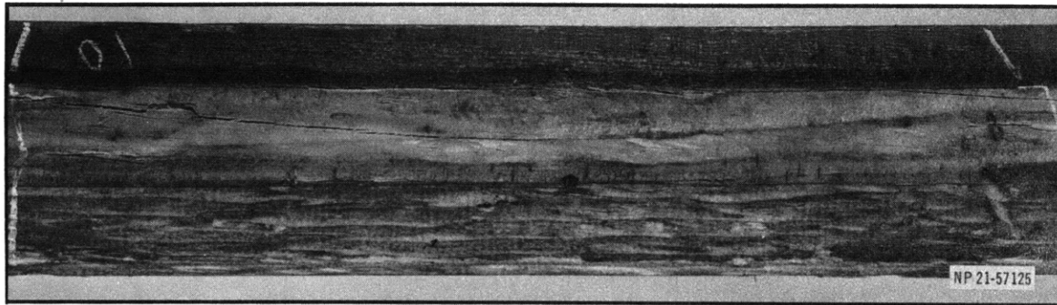
Figure 27 – Portion of Flight-Deck Planking Removed from Test Position 10 after Deck Reaction of 66,000 Pounds with F 2 H-3 Landing Gear
