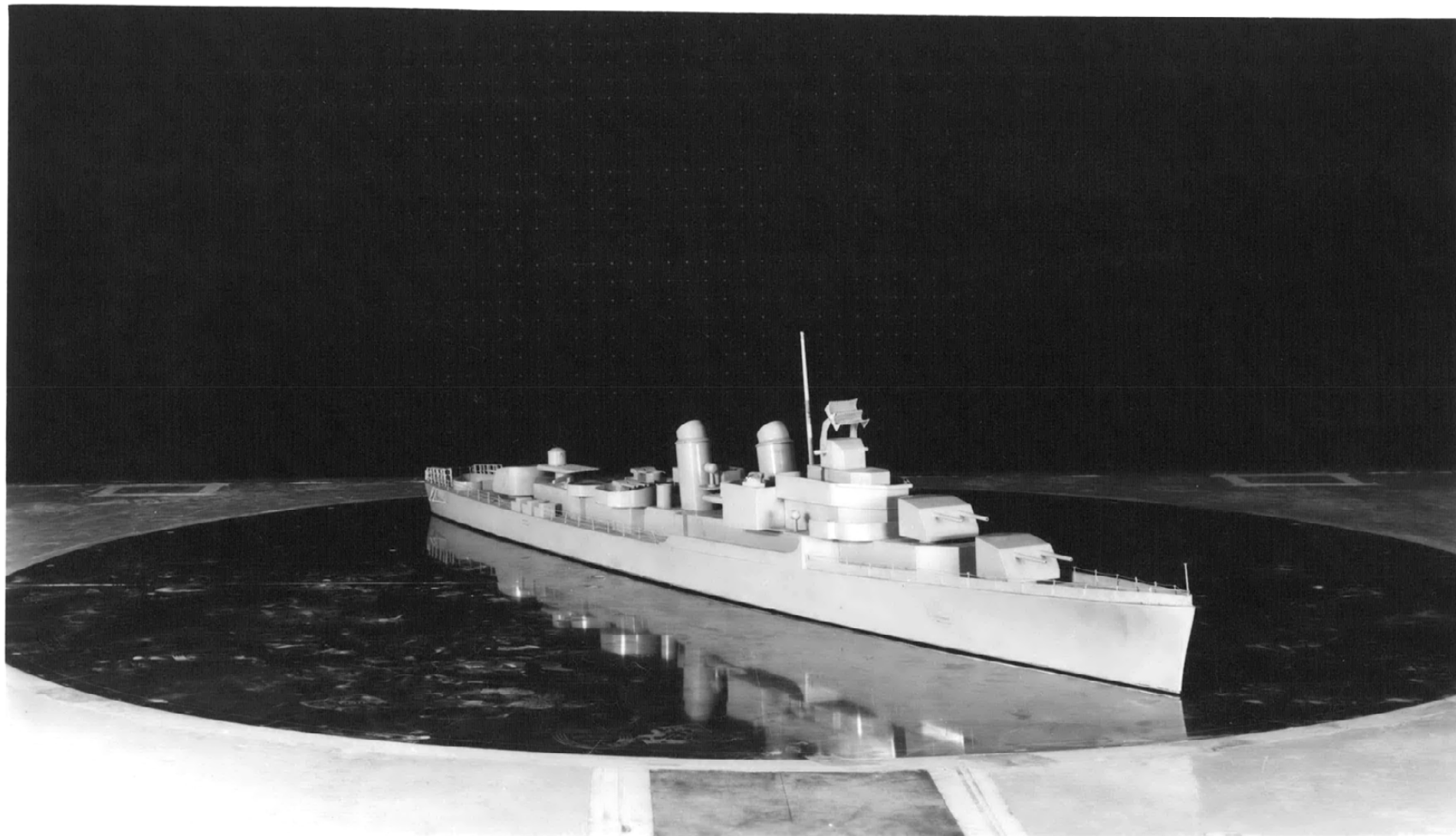
Figure 2 - One-Quarter Starboard View of a 1:73.8-Scale Model DD692-Class Destroyer Mounted on Ground Board in Wind Tunnel
