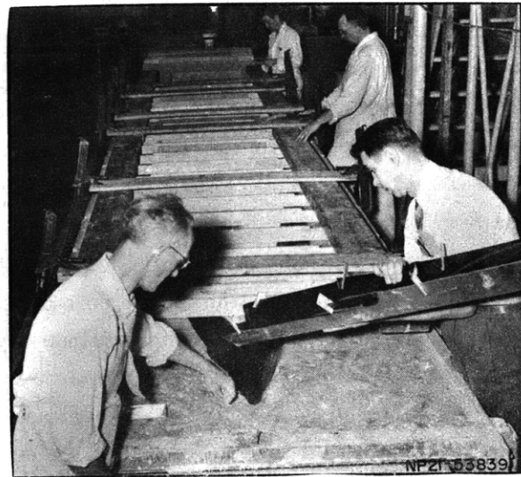
Figure 7 - Preparing for Pouring of Wax for 20-Foot Model
