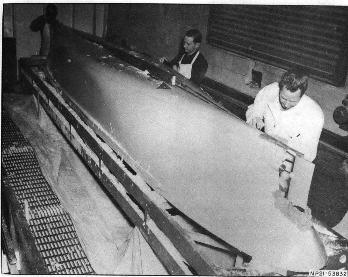
Figure 14 - Final Scraping on a 20-Foot Model
