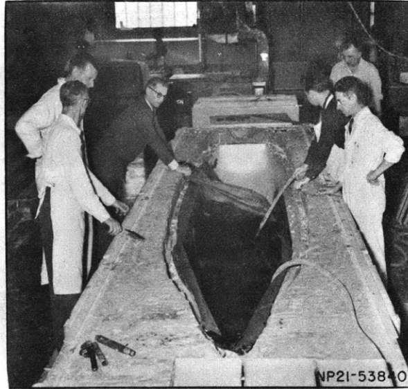
Figure 9 - Removing Rubberized Cloth from Model
