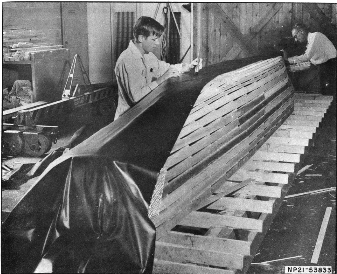
Figure 4 - Fabrication of Core for a 20-Foot Wax Model
