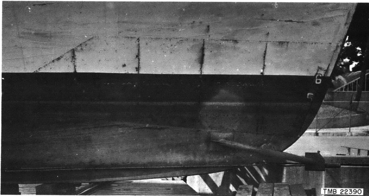
Figure 3 - View of EMS-1 Showing Bow Log
