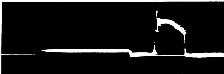
Figure 7 - Sample Oscillograph Record of Specimen 1N6 showing Load plotted on a basis of Time during Elongation
